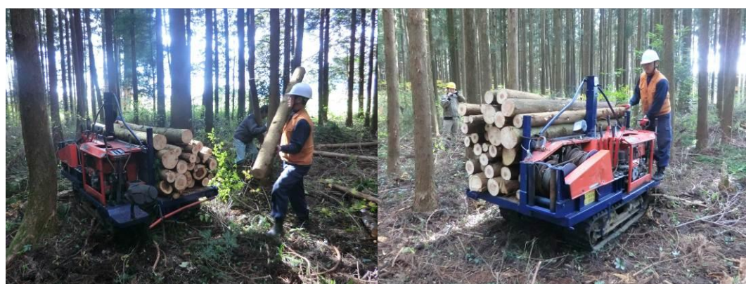
Photo 2: Forwarding operations by a private logging contractor
