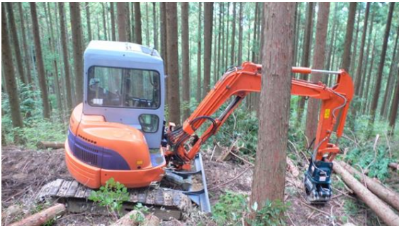
Picture 1: Grapple with winch (bucket capacity 0.16m 3 )
