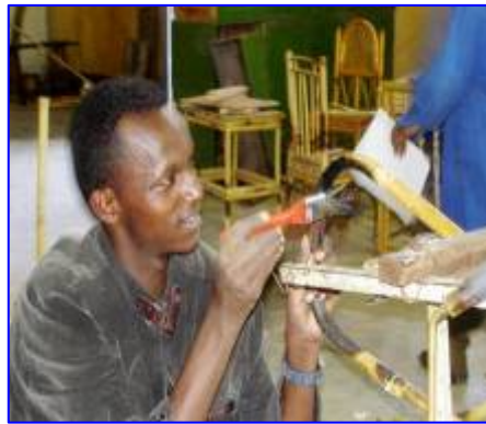
Curing Bamboo with Fire
