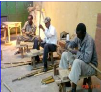
Making the Bent Mortise for Bamboo Furniture
