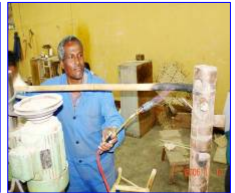
Straightening Bamboo with Fire
