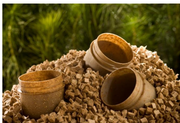
Woodfibre dice (Woodforce) used for making natural fibre-plastic composite products and hot-fill cosmetic pots made from PLA and wood flour. Scion photograph
