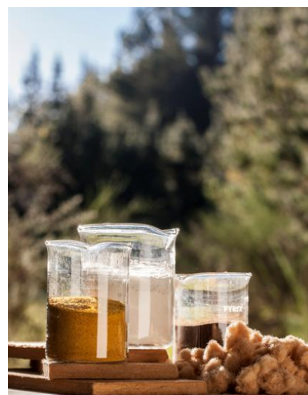
Ingredients for a 100% biobased adhesive (Ligate™) that can be used to make plywood with very low VOC. Scion photograph
