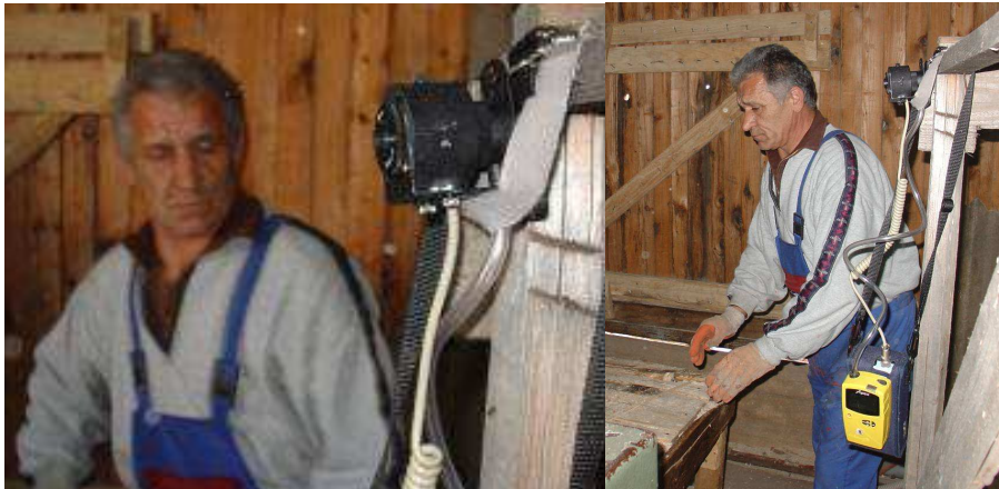
Figure 2 – Photometry unit stationary located near the workplace
