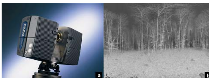
Figure 1: (a) laser scanner Faro Photon 120, (b) a 44 million points scan quick view
