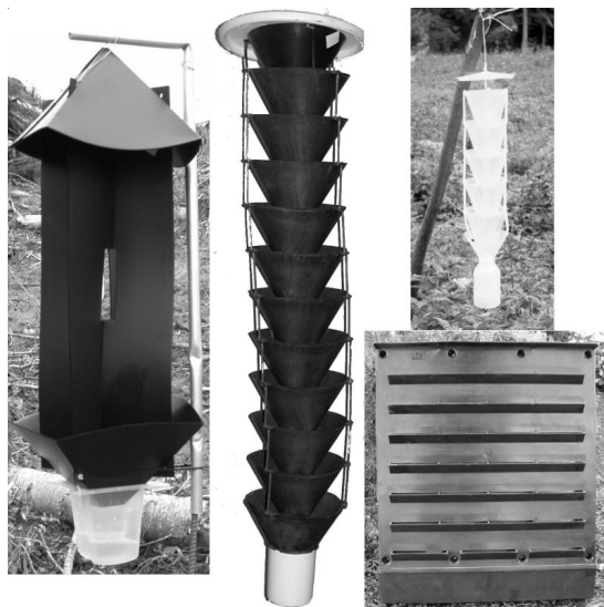
Figure 1.—Intercept PT (left), Multi-funnel trap (center), IBL-3 trap (top right), Theyson trap (bottom right).
