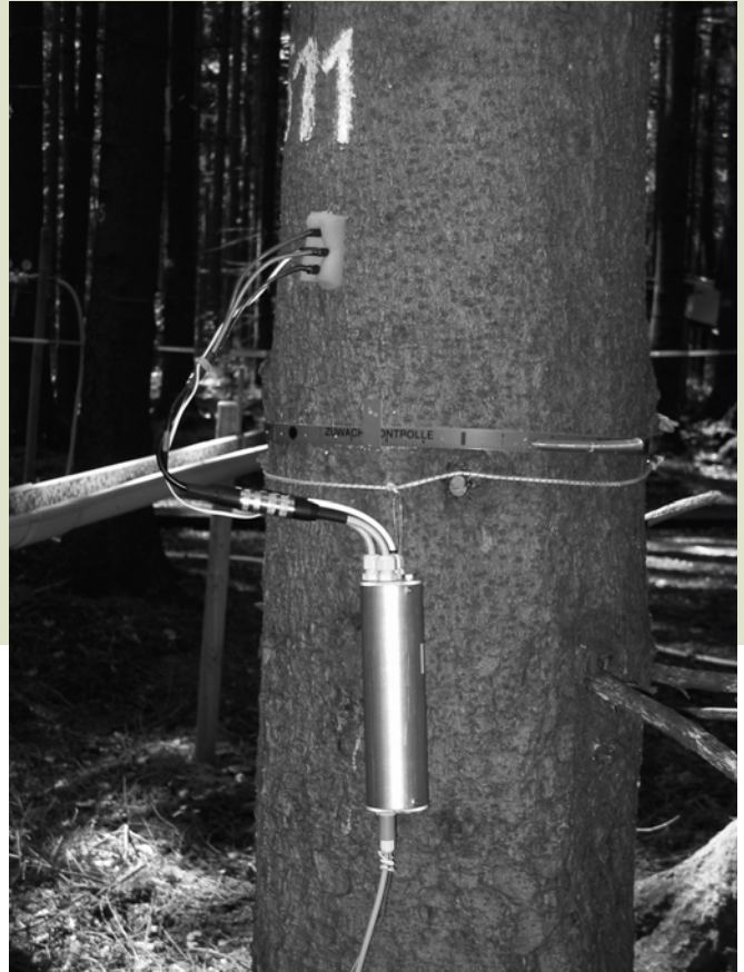
Photo: Sap-flow measurements for the calculation of crown-level stomatal ozone flux in Norway spruce (provided by IUFRO RG 7.01.00)
