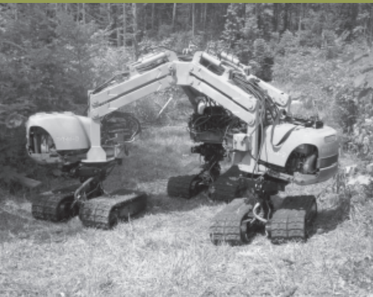
Photo by of Hans Heinimann, ETH Zurich, Switzerland: Tree planting machine, Furano area, Hokkaido
