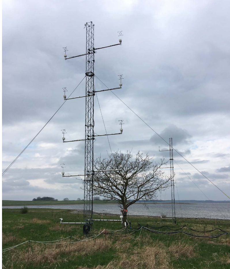
Oak tree at Risø campus, Roskilde, which is monitored for movement in the wind. Masts are instrumented with sonic anemometers to measure the flow in front of and behind the tree. Photo by Barry Gardiner
