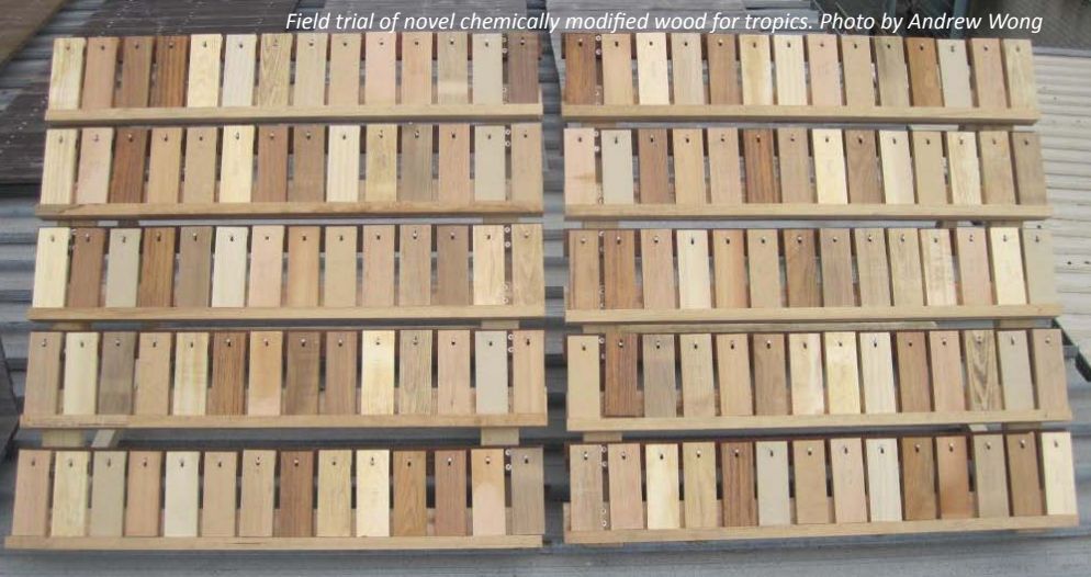
Field trial of novel chemically modified wood for tropics. Photo by Andrew Wong
