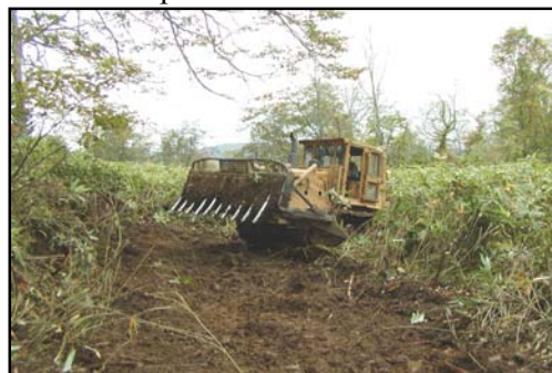
Fig.3: Scarification by a bulldozer for natural regeneration.
