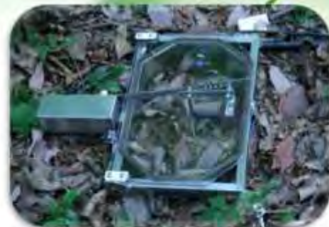
(AOCC ; Automatic Open/Closing Chamber system)
