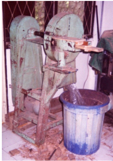
Fig. 1: Disc flaker which converted wood billets into strands
