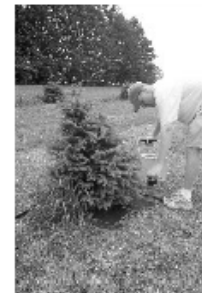
Figure 7 (Right): Measuring volumetric soil moisture using a portable TDR system.
