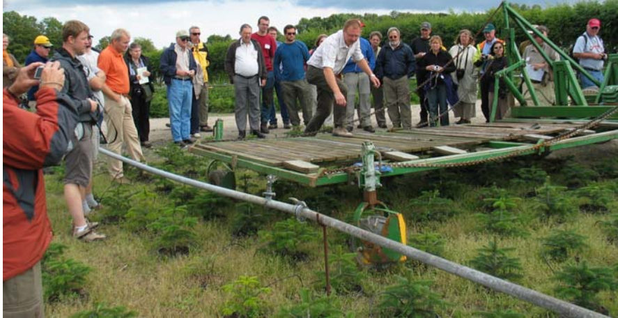
Ulrich Gejl demonstrates machinery used for shaping of young trees in pots.
