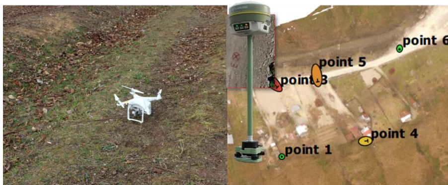
Figure 4. An example of GCP surveyed (right) and DJI Phantom 3 model UAV system (left)
