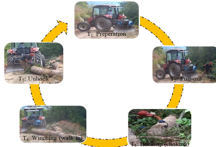
Figure 3. Main work elements in a cycle during winching operation with tractor
