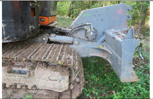
Figure 2: lateral view of the winch attached to the excavator's blade
