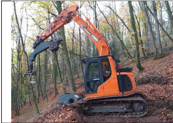
Figure 4: TVS20 mounted on a 14-ton excavator, winch on the front blade, hub in grapple configuration at the end of the boom
