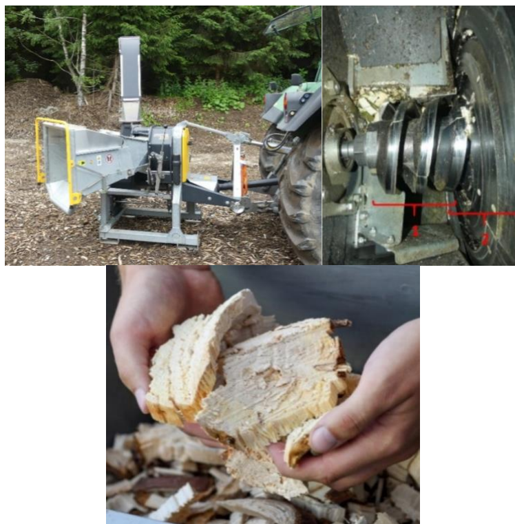
Figure 5: left: The Effiter 20.30 duplex-spiral chipper powered by a conventional farm machine; middle: Duplex spiral of the Effiter 20.30 with the cylindrical screw on the left (1) and the flat screw on the right (2) as seen from the inspection hatch; right: Effits from stemwood of Norway spruce (photo: Tobias Hase, StMELF)
