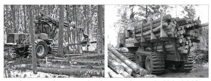
Figure 3. Left image: Harvesting machine processing a tree into logs in a thinning operation. Right image: Forwarder at the landing with a load of logs.
