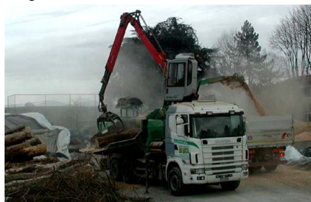
Figure 1. Examples of typical industrial operation: chipper truck and truck-mounted chipper steered by a single operator sitting inside the enclosed cab
