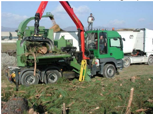
Figure 1. Examples of typical industrial operation: chipper truck and truck-mounted chipper steered by a single operator sitting inside the enclosed cab
