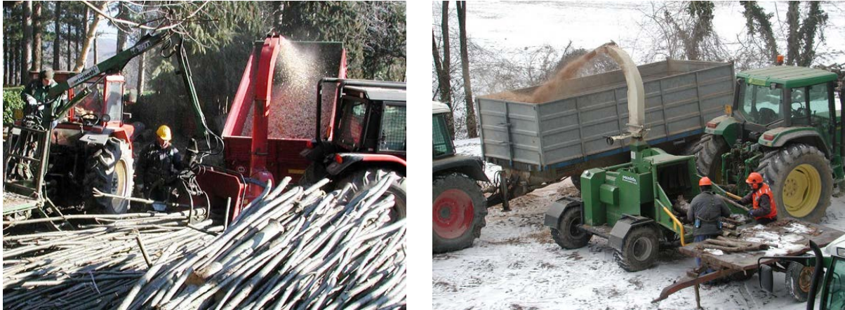
Figure 2. Small-scale chippers fed manually or by hydraulic grapple
