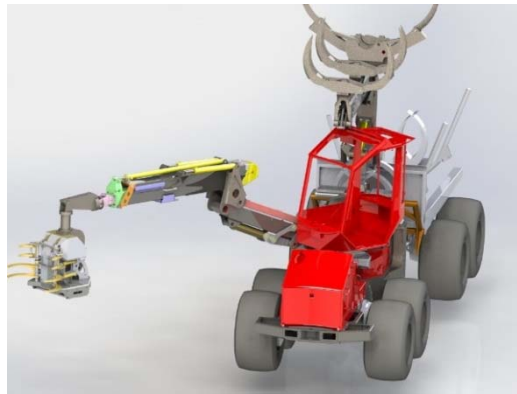
Figure 1: CAD-drawing of machine concept, Cintoq
