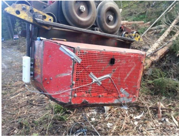
Figure 1: Konrad Woodliner carriage with access point facing the tower, android device and single board computer - raspberry pi at the bottom with attached camera.
