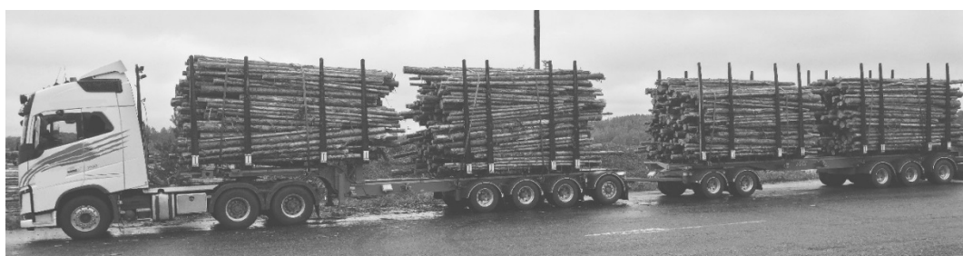
Figure 1: One of the HCT trucks studied, a Volvo FH16 with 750 hp (559 kW). Truck + semitrailer + drawbar trailer. The length is 30.5 m. It is actually designed for 102 tonnes, but for the designated routes the maximum allowed GVW is 94 tonnes. (Photo: Bo Dahlin)
