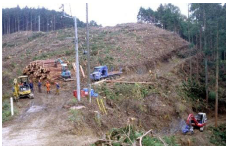
Figure 1. Cut-to-Length (CTL) system on a steep terrain leaving logging residues on forest land.
