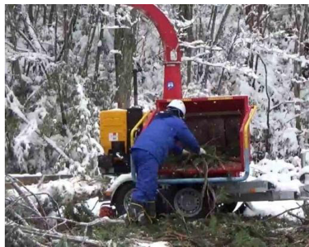
Figure 3. Manual chipping of logging residues by using TP250 mobile turnable chipper.
