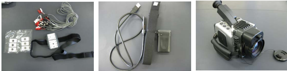
Fig. 3 MARQ16(left)、HEXOSKIN Heart rare monitor(center)、Thermographic camera(right)
