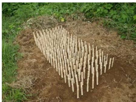
Photo 4: Outdoor exposure test site for Moso bamboo sticks
