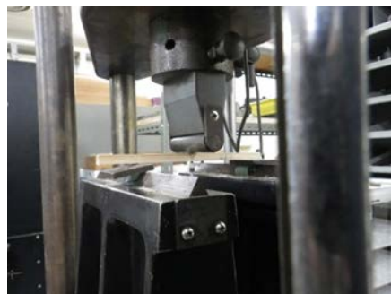
Photo 5: Snapshot of bending test
