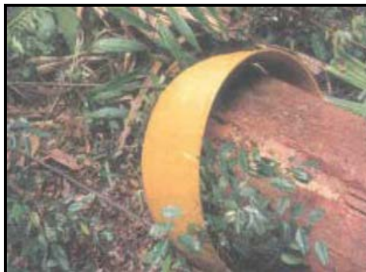
Figure 7. An ECOLOG fiberglass cone fixed in front of log to assist hauling process.
