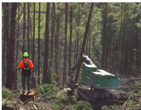
Figure 2. Field testing of remotely controlled winch-assist felling machine in New Zealand (Milliken and Wood, 2016)
