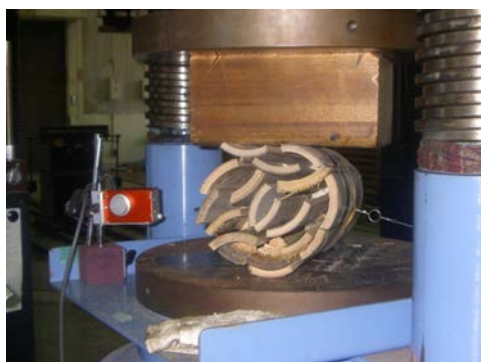
Photo 6: Snapshot of load test of a bundle of bamboo sticks
