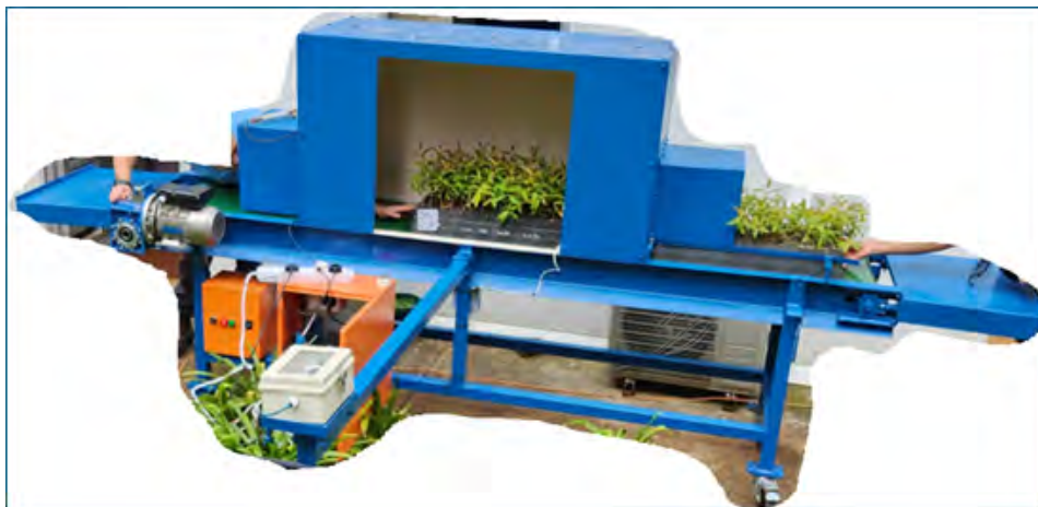
Figure 1: Sappi's smart computer vision mechanical photobooth that can automatically measure plant quality in a commercial nursery.
