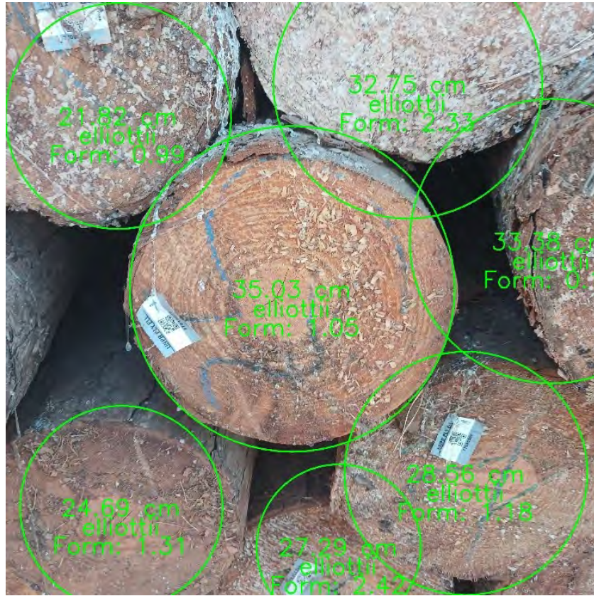
Figure 1: Example of AI-based log species classification and diameter measurement using YOLOv8. The bounding boxes and labels indicate detected log species and their respective diameters.
