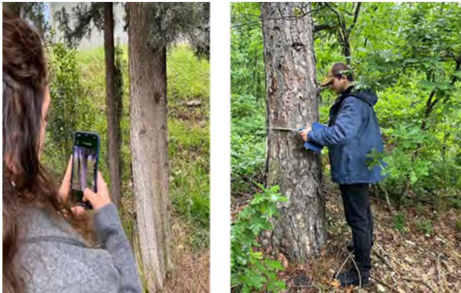
Figure 3: DBH measurements using smartphone (left) and clipper (right)
