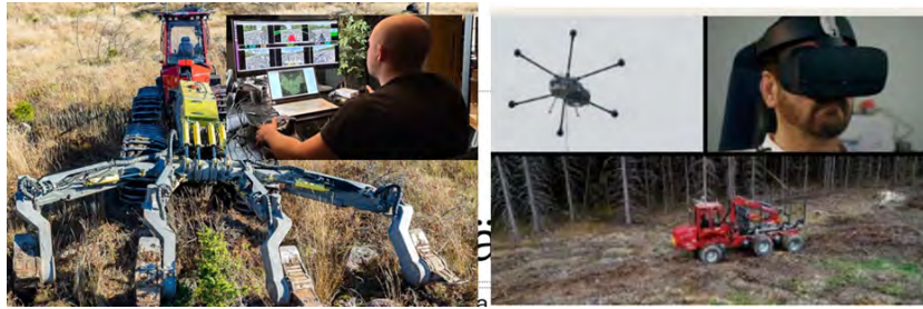
Figure 2: Left, tests with remote controlled operated moulder, Bracke 4-row moulder on a large Komatsu forwarder. Right, tests with remote controlled forwarding operation, communication via commercial 5G and a drone for amplifying the 5G signal at the rural logging site. Distance between operator and forwarder approx. 150 km.
