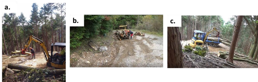
Figure 6: Loading and transport. Loading with a grapple ( a. ), once with a mini-forwarder ( b. ), and three times with a forwarder ( c. ) for logs of 3.72 m 3 to the landing.
