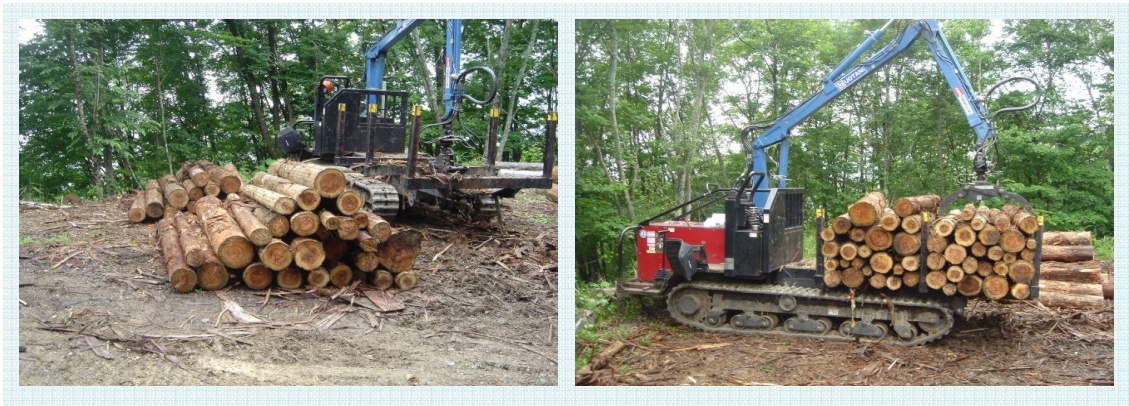
Figure 1: Log handling work with Grapple Loader
