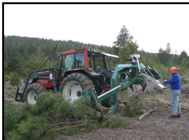
Image 6. Tractor with processor attachment.
