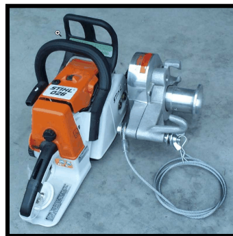
Image 4. Chainsaw powered capstan winch.
