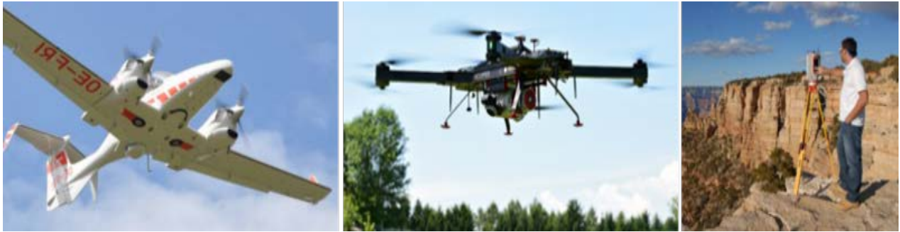
Figure 1: LiDAR Acquisition Platforms: Fixed Wing Aircraft, Unmanned Aircraft, Static Tripod
