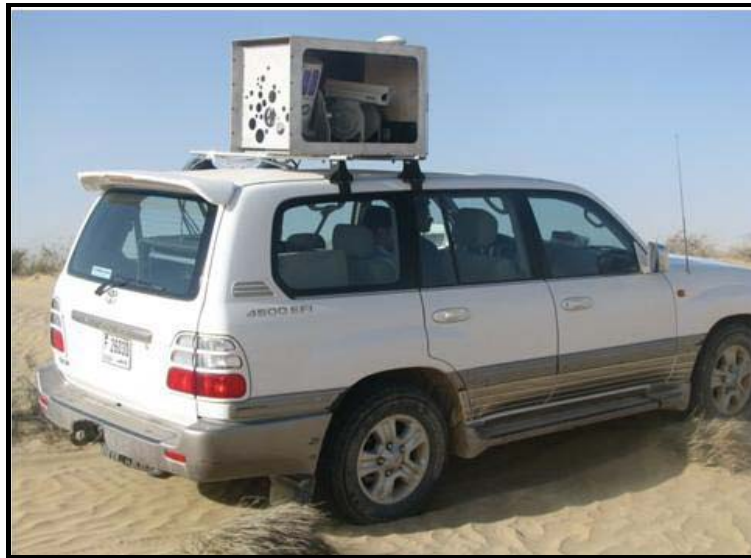
Figure 3: Dubai World, Limitless Dynamic Laser Scanning System equipped with IMU and GPS.
