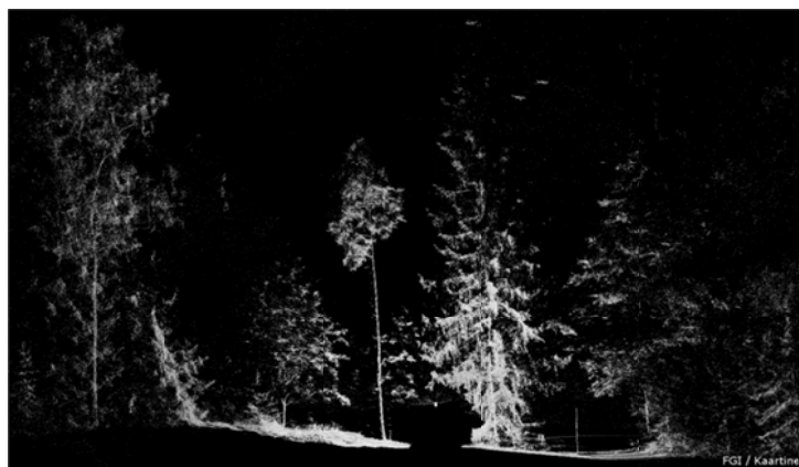
Figure 1. Representation of a point cloud collected with MLS from study area. Trees are well characterised.
