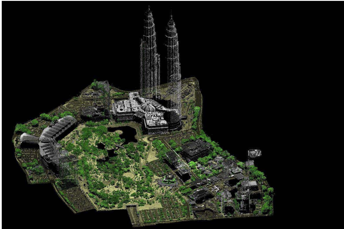
Figure 2: LIDAR color coded point cloud of the KLCC showing world's tallest twin building in Kuala Lumpur (451.9 m).
