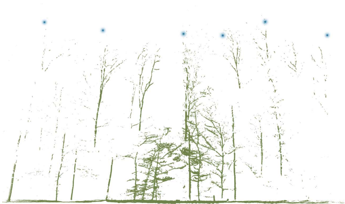
Figure 3 View through TLS-point cloud (green) with a depth of 1.5[m]. The blue points represent the ALS-trees found by Gupta et al. 2010
