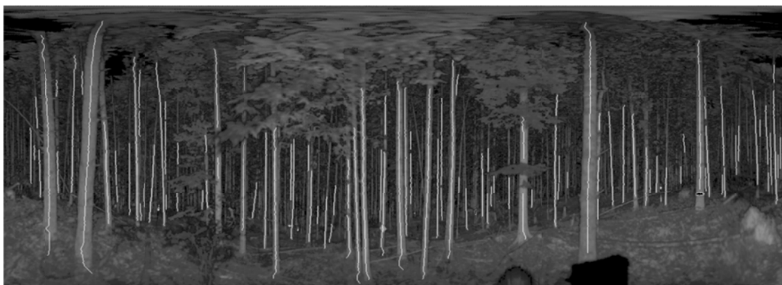
Figure 2 Automatic tree detection from range image data. Shown in bright white is the Medial Axis Transformation, filtered using the parameters \rho , \zeta , and n .
