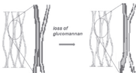
Figure 1: Schematic picture of the increase of cellulose aggregate size resulting from extraction of glucomannan. The increased size is the result of a larger area of contact between adjacent aggregates/fibrils, making on average larger aggregates in cross sections to be viewed.
