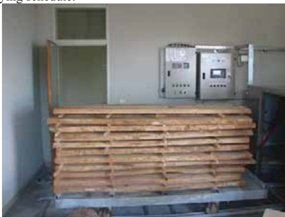
Figure 6. Outlook of dried lumbers with non-protective drying schedule.
