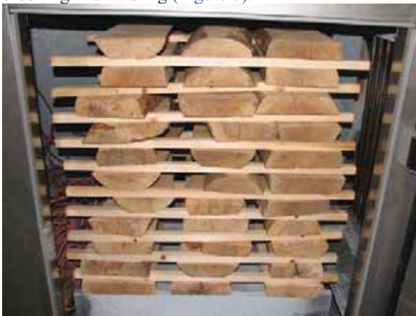
Figure 6. Outlook of dried lumbers with non-protective drying schedule.
