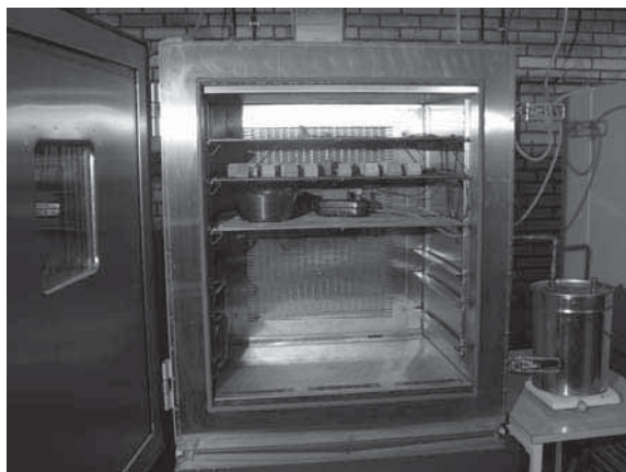
Figure 2. Small clear wood samples in laboratory cabinet. Saturated conditions were guaranteed by means of constant supply of vapour from an external boiling pot. Power rate exceeding 2 MW/m 3 . From (Landel, 2004).
