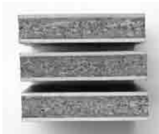
Figure 2. Test specimens after 24 hours immersion in water
