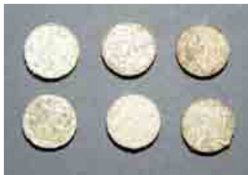
Figure 4. View of tablets for determination of ash content, sulphur and high calorific value of briquettes made by different raw material
