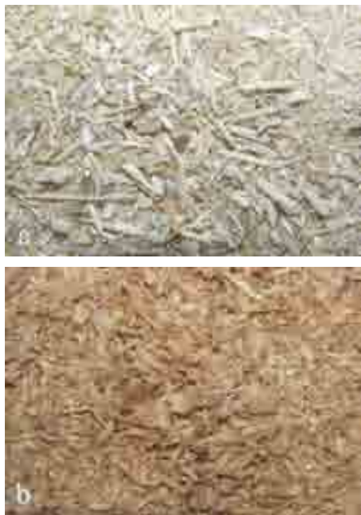
Figure 3: View of chipped raw material for production of briquettes a-corn stems; b-beech wood
