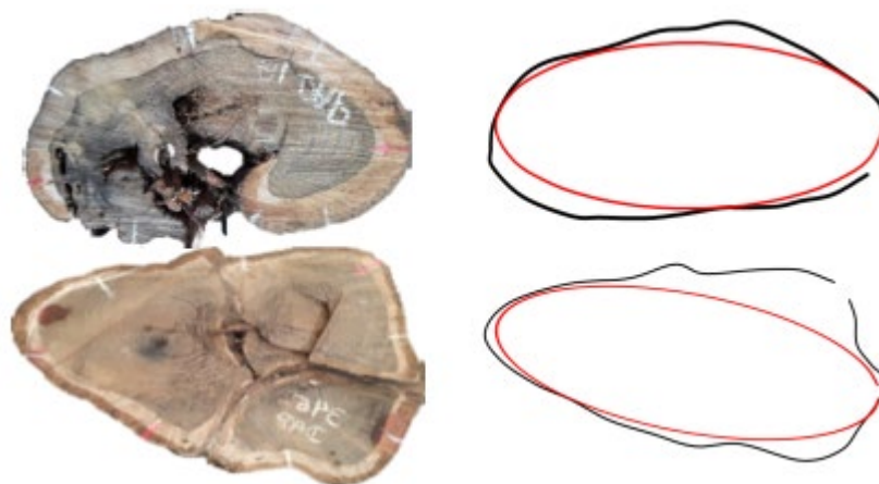
Figure 1- Example of irregular trunk outline in tree species used in urban areas (on the left) and representation of the real outline (in black) and generated from an elliptical outline generator (red) on the right.
