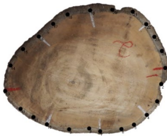
Figura 1- Plotting of the outline points on a photograph of the surface of the wooden disk to obtain the real outline coordinates.
