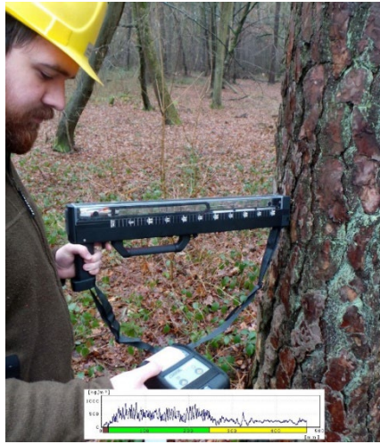
Figure 8. Electronically regulated resistance drilling in a standing tree using a Resistograph® tool (Photo credit: Frank Rinn).
