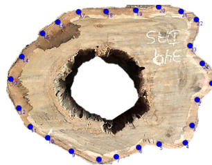
Figure 1 - Example of an image with the points already demarcated to obtain the outline.
