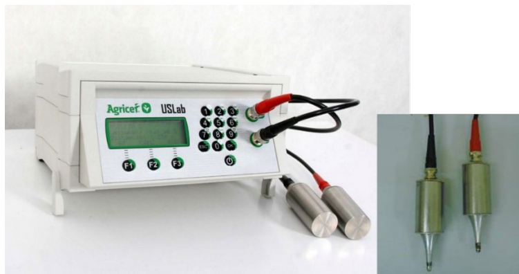
Figure 2 — Ultrasound equipment and transducers adopted in our research
