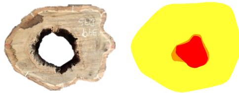
Figura 7 - Example of an image generated with 3 colors considering the cut velocities for inference of Ca (up to 40%) and Ca+Bio (up to 45%) and filtered
