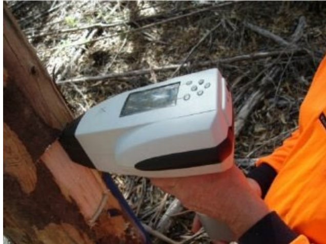
Figure 3. NIR acquisition on standing trees using a handheld device (Meder et al. 2010. Photo credit: Roger Meder).
