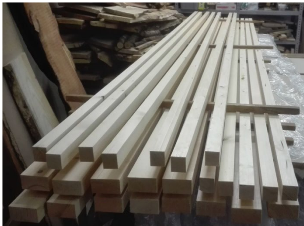
Figure 1 — Selection of small size- ( 42 \times 42 mm) and large size ( 42 \times 84 mm) test specimens with for the investigation of dynamic mechanical properties.
