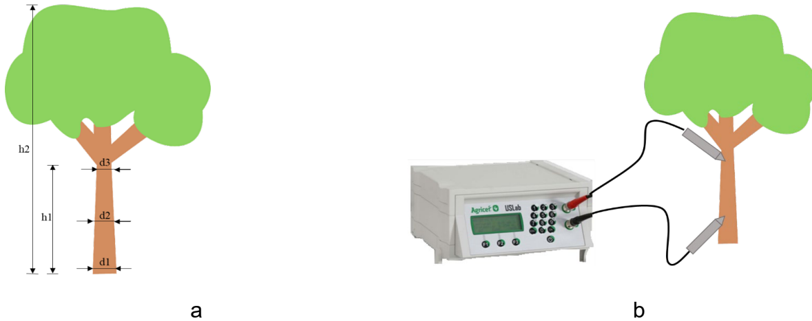
Figure 2. Dimensions obtained from the plant (a) and scheme of the ultrasound test performed on the clones (b)
