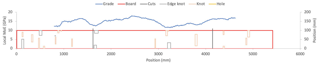
Figure 2 —Example board MoE profile and defect data
