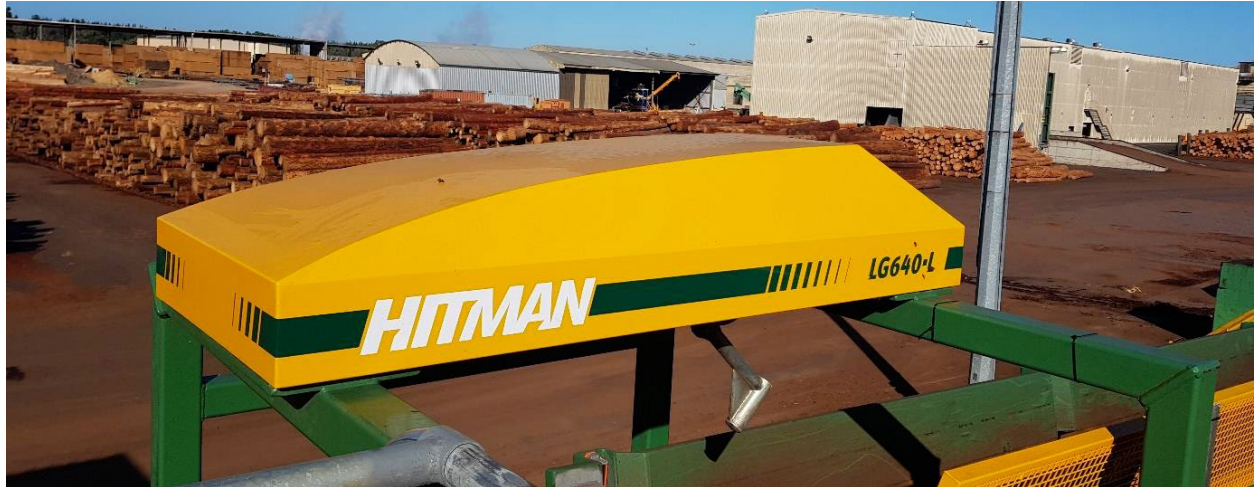
Figure 3 Hitman LG640™ installed on log chain in MSG log processing facility
