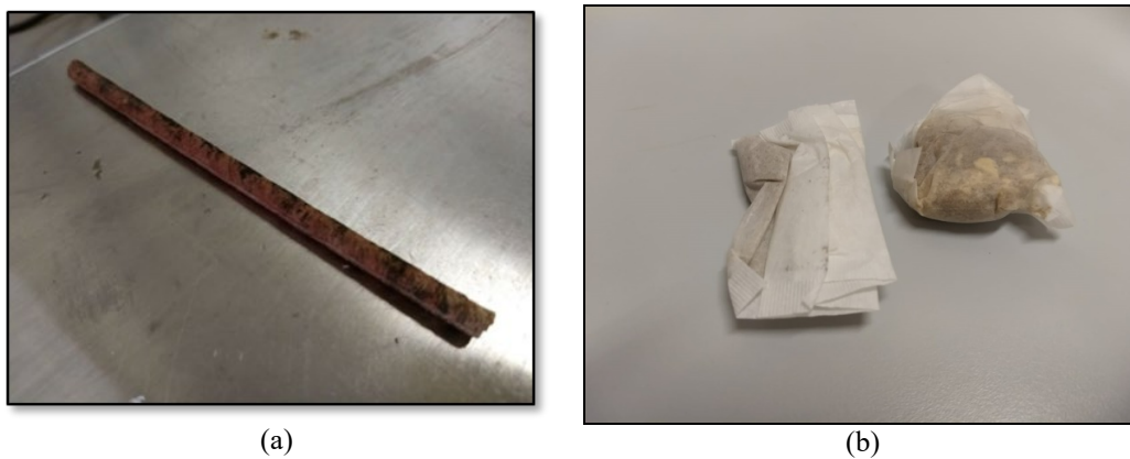
Figure 2 — Specimen obtained by a. Increment borer and b. WoodEX
