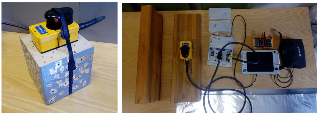
Figures 5 and 6 —Antenna on beech specimen and Scots pine, respectively.
