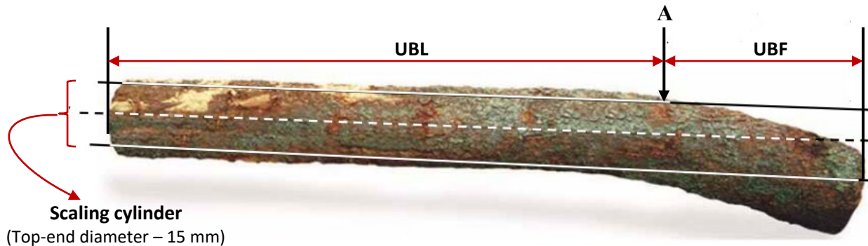
Figure 1 – Graphical representation of the “loss of saw yield” principle.
