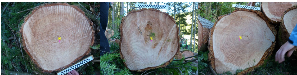
Figure 4 — Some worst cases where our method fails to detect precisely (less than 5mm) the pith. In red cross results of the first step, and in yellow star the results after the second step. Errors can be explained by a high presence of sawing marks, knot near the pith (third image). The first failure can be explained by the cross-section outline that is not circular.
