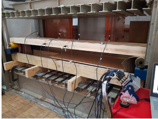
Figure 1 —CLT panel instrumentation for operational modal testing.
