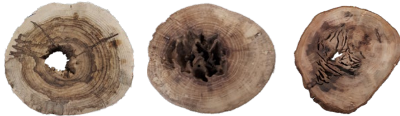
Figure 1 – discs with different types of deterioration.
