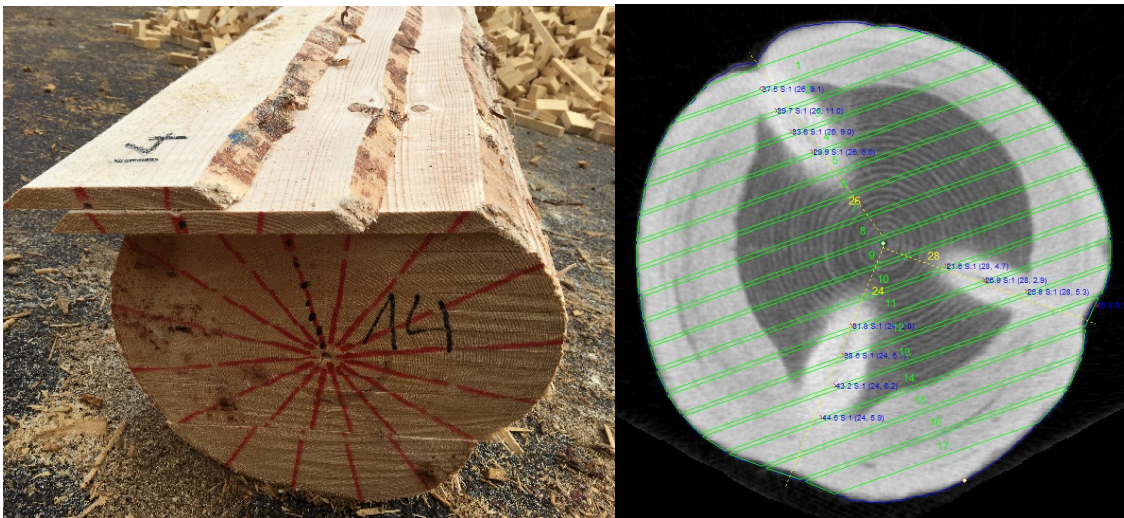
Figure 5 — An example of reference taken on a log that is CT-scanned and then sawn in boards (left), the manual measurements superimposed on the CT image (right).
