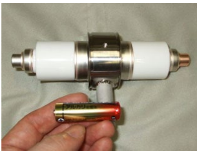
Figure 1 —High-energy pulsed X-ray source has developed by Suzuki in 2008.
