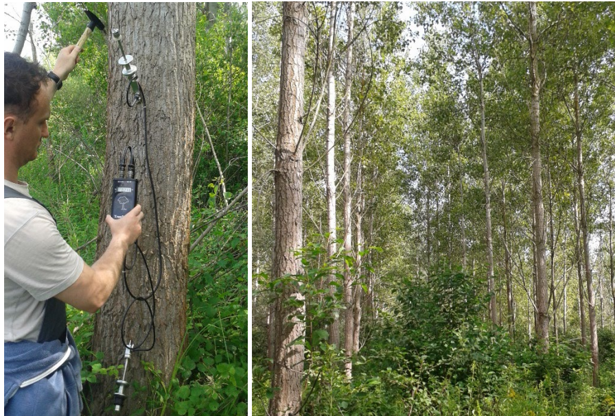
Figure 2 — Measuring with “Fakopp” TreeSonic device (left); spacing of Újrónafő 11G platntation (right)
