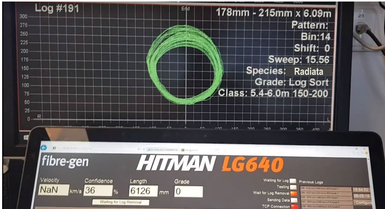
Figure 4 LG640 and USNR Scanner user interfaces showing length outputs
