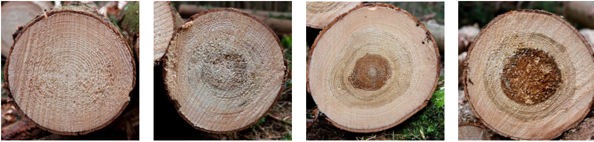
Figure 1 —Cross sections of spruce trunks with rot grades FG 0, FG 1, FG 2, and FG 3 (from left to right)
