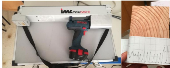
Figure 4. IML RESI F-400S inspection drill and result of inspection with drill on a conifer [Coba, 2018].
