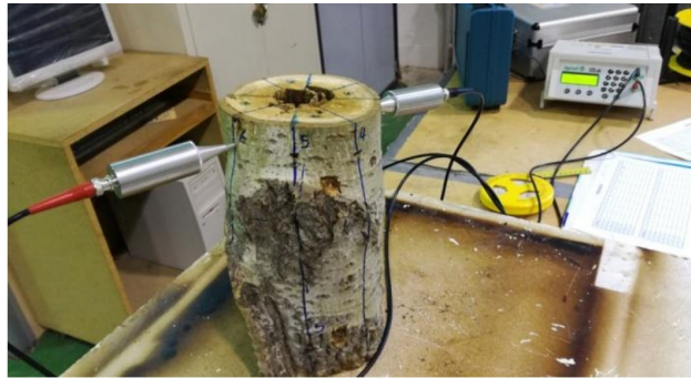
Figure 2. USLab ultrasound equipment and log marked in sections [Coba, 2018].
