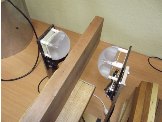
Figure 1 —Picture and schematic representation of the measurement system, including the focusing lenses on the sensors.
