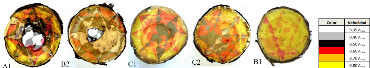
Figure 8. Tomographs of the cross section of the logs [Coba, 2018].
