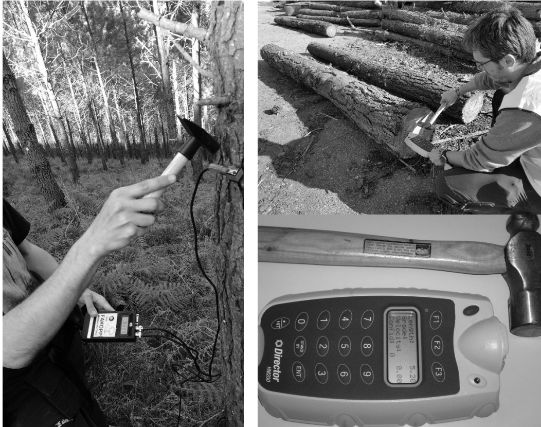
Figure 1 - NDT measurements: standing trees (MicrosecondTimer, left), logs (Fibergen Hitman HM200, upper right) and Hitman HM200 (lower right)
