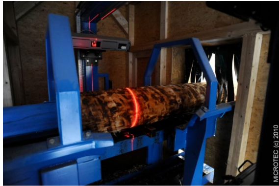
Figure 1 —3D-laser scanner at the entrance of a saw mill
