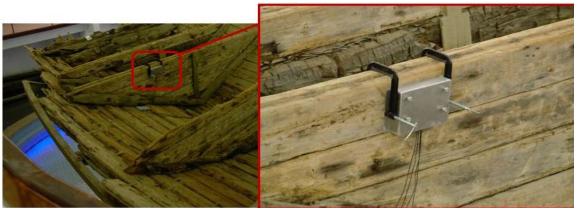
Figure 1. Four acoustic emission sensors coupled to the partition during on-site monitoring of the wooden object
