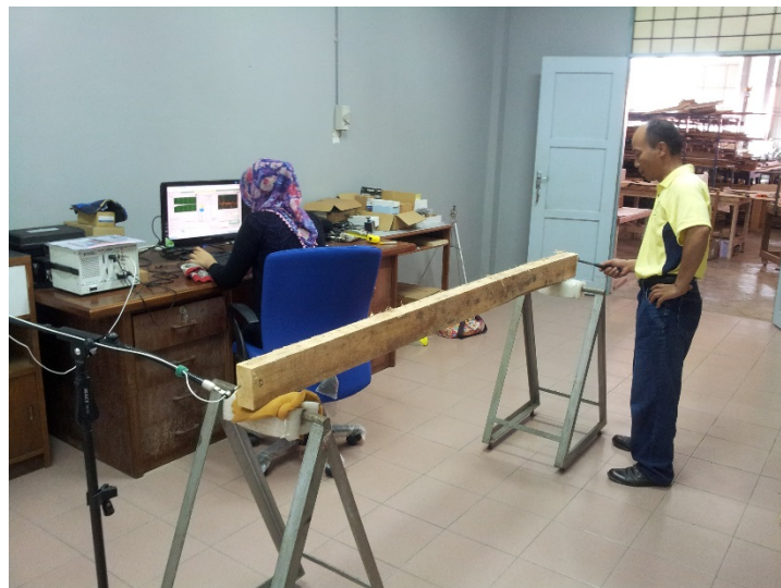
Figure 1 — Nondestructive testing using MOE Evaluator
