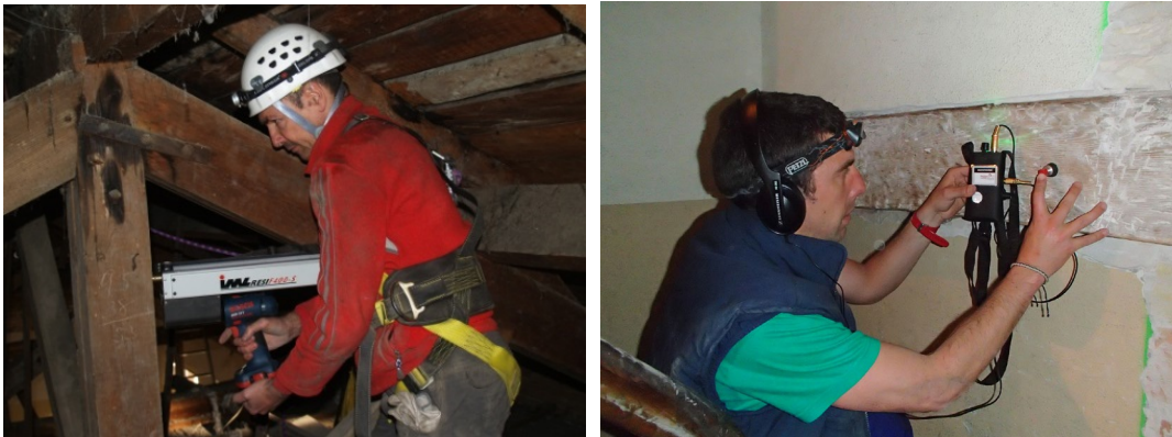
Figures 3 and 4—Resistograph device and termite detector.
