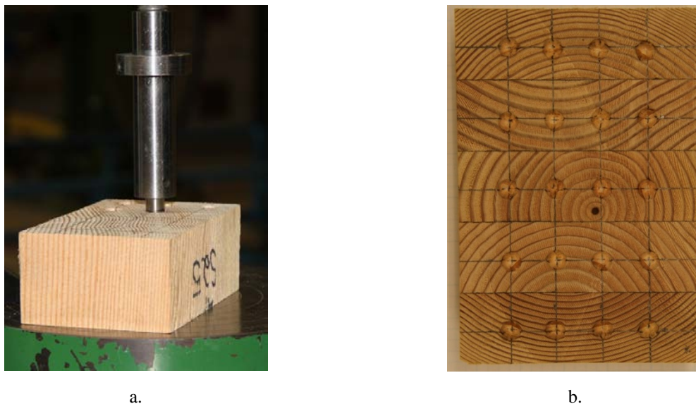
Figure 3. Janka hardness testing: (a) sawn timber remnant undergoing Janka hardness test; (b) hardness test impressions across glulam remnant cross section.
