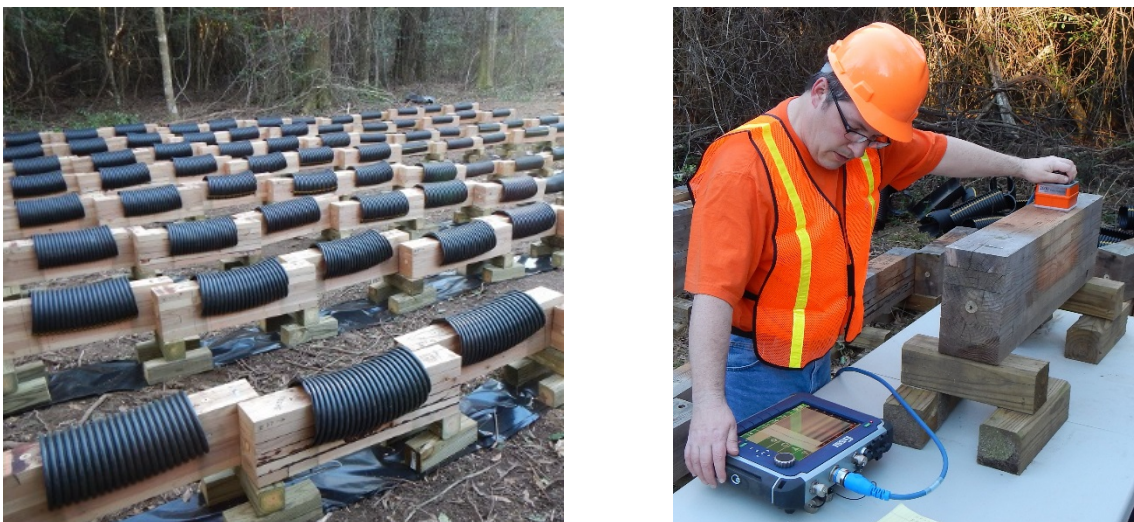
Figure 5. Specimens as positioned on site, and GPR scanning of specimens.
