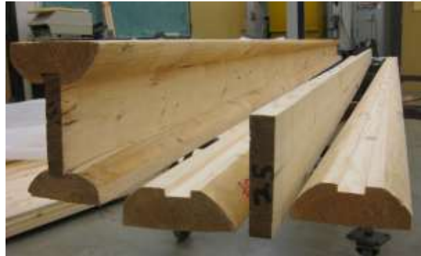
Figure 2 -- Machined components prior to gluing. The groove cut in the flanges was made to assist with positioning the webs during assembly.
