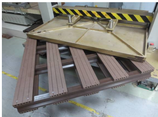
Figure 5 —Measure WPC pallet sample in Compression tests
