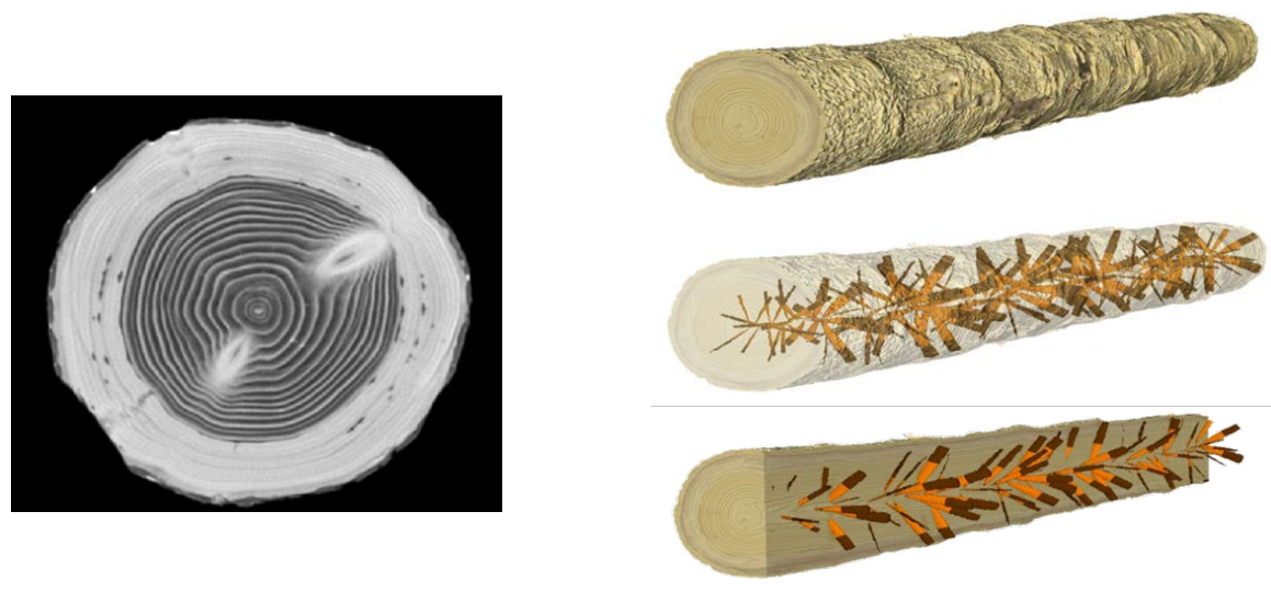
Figure 5 —Roundwood sawing optimisation according to X-ray based computed tomography; (Bruechert et al. 2017)
