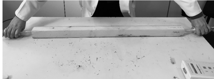
Figure 2 – Direct ultrasonic stress wave measurement
