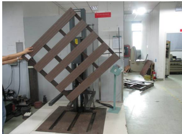
Figure 11 —Measured WPC pallet sample in free-fall drop tests.
