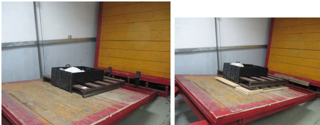
Figure 14 —Measured WPC pallet sample in incline impact tests on pallet deck edges, blocks or posts, and stringers.
