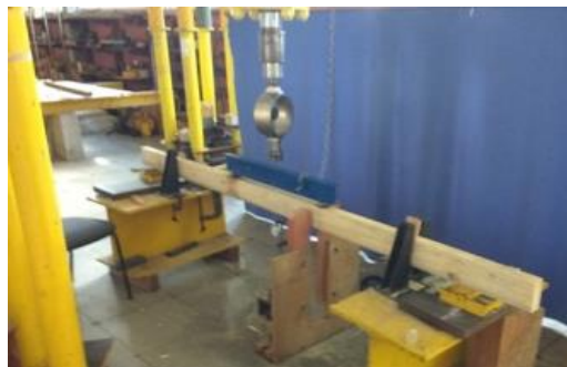
Figura 2 —Static bending test to determine edgewise modulus of elasticity (MOE)
