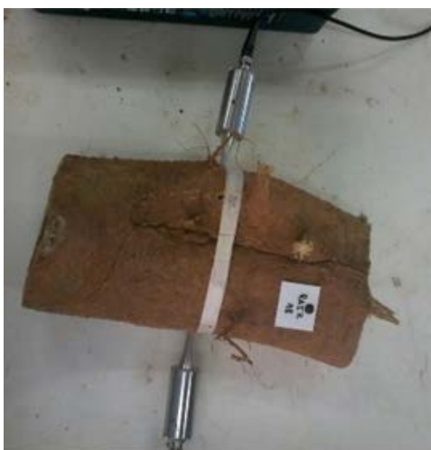
Figure 3 —Example of ultrasound test in a wood specimen from root .
