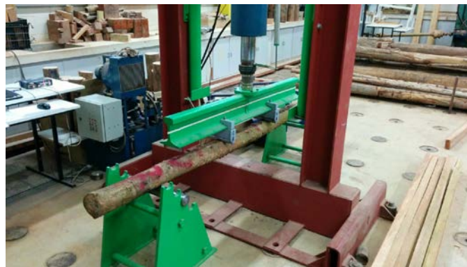
Figure 3. Static bending test in logs
