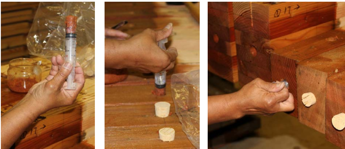
Figure 4. Inoculating specimens with Fomitopsis pinicola , brown-rot.
