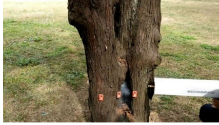
Figure 9 —This figure caption is Resistograph® experiment with smog, smog rised by micro-drilling testing.
