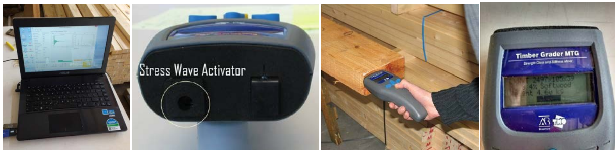
Figura 1 —Portable device Brookhuis Microeletronic Timber Grade (MTG)
