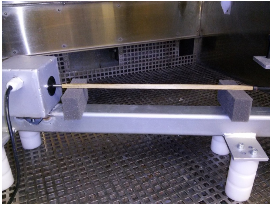
Figure 1. The experimental setup inside a climate chamber. The sensor on the left is a capacitor type extensometer. The specimen is placed on rubber foam. A steel frame is holding the extensometer, sample and the reference point on the right.
