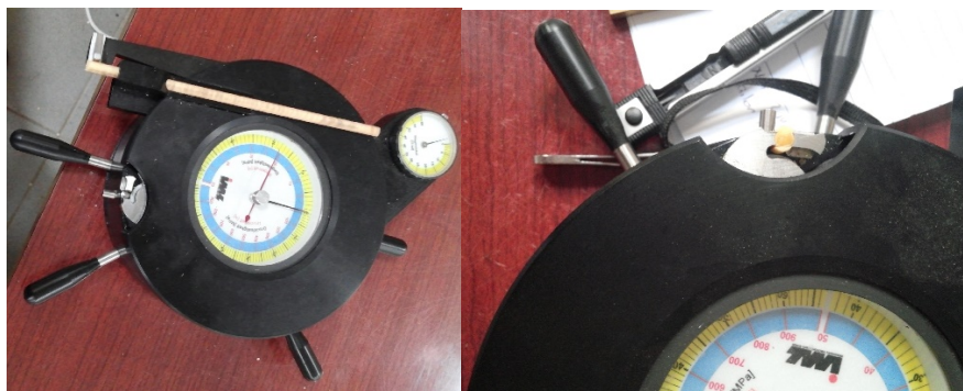
Figure 3 — Experimental setup for radial bending (left) and compression parallel to grain (right) test on the increment cores.
