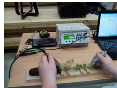
Figure 2. Ultrasound test in Eucalyptus (a) and Pinus pinaster (b) seedlings
