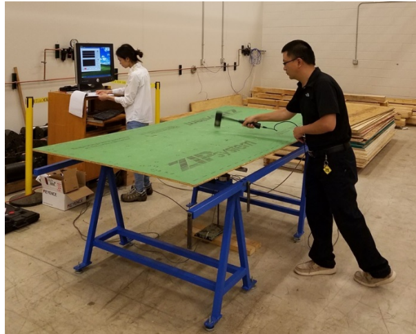
Figure 4 —Vibration test of a full-size OSB panel
