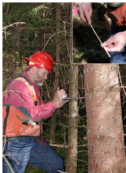
Figure 1. Increment borer being used to extract a core sample from a standing tree at breast height.
