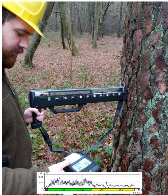
Figure 4. Electronically regulated resistance drilling in a standing tree using a Resistograph tool (photo credit: Frank Rinn).
