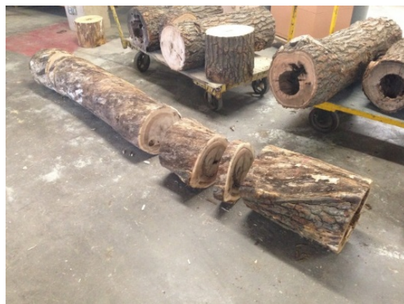
Figure 3 —Dissected log sections revealing internal defects.
