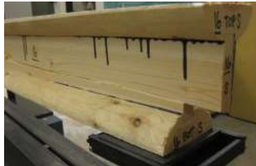
Figure 6 -- Seven of the 28 I-beams tested to failure in bending exhibited shear failure in the webs.
