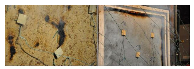
Figure 3: Differences in integrity fail for 50 WB (left) 100 WB (right)
