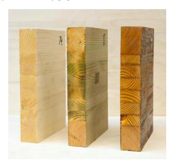
Figure 1: Examples of tested 44x200x200 mm glulam specimens. From the left: untreated, CC-impregnated, and pine oil impregnated. The material from small sized timber was mainly sapwood which can be seen as high penetration of preservative liquid in the inner lamellae of the CC-impregnated specimen, whereas virtually no preservative has penetrated in the surface lamellae that were made of larger logs with higher proportion of heartwood. (Photo: Erkki Oksanen, Metla)
