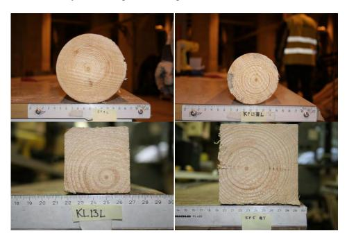
Figure 1: Examples of the round (80 and 120 mm) and square (50×50 mm and 100×100 mm) post specimens.
