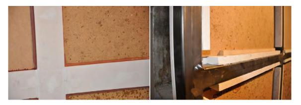
Figure 2: Fire test preparation (left: flame exposed, right: flame averted)
