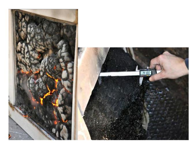
Figure 7: Foaming of 50 WB panel (left) and foam thickness of 100 WW (right)
