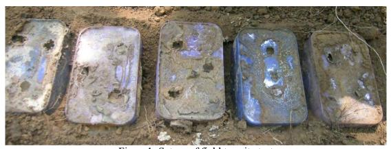
Figure 1: Set up of field termite test
