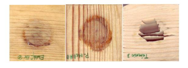
Figure 4: Attacked area of the treated wood (*Pinus sylvestris*) exposed to termites according to EN118 2005 (Dose applied: 10 mg/cm<sup>2</sup>)
