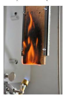
Figure 1: Procedure of small flame test
