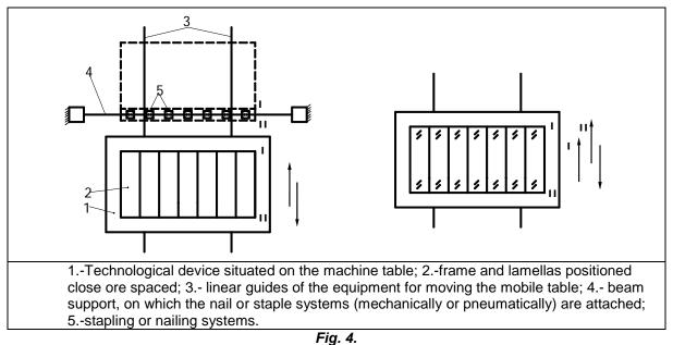
Scheme for equipment of applying reinforcement accessories (nails or staples).
