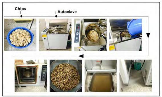
Fig. 2. Hydrothermal treatment of chips.
