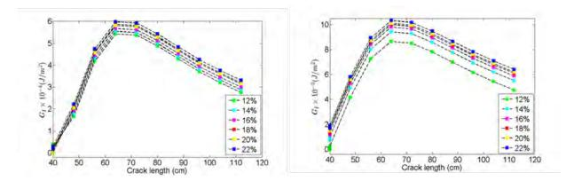
Fig. 4. Effect of variation in moisture content (MC) on energy recovery rate (G) versus crack length:  $\Delta T = 10 \ ^{\circ}C (a), \ \Delta T = 30 \ ^{\circ}C (b).$
