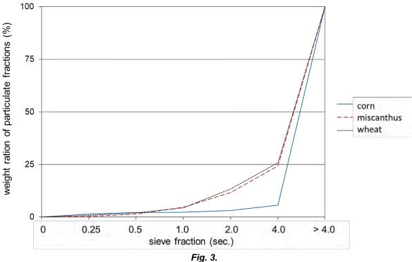
Weight parts of the residues from different plants per particle fraction.
