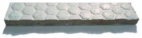
Fig. 9. Surface coating of imprinted pattern particleboard.
