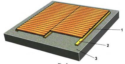
Fig. 2. Type A Panel Structure 1 – beech wood parquet frieze; 2 – resinous wood beamlets; 3 – concrete support layer.
