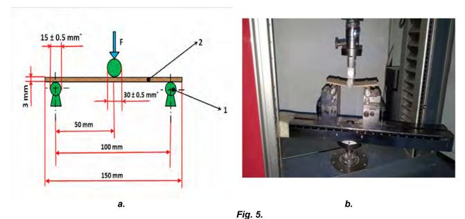
Determination of the bending strength and modulus elasticity in bending of HDF panels: a-principle, with 1-supports; 2-test piece; F-loading force; b-ZWICK 010 testing machine.
