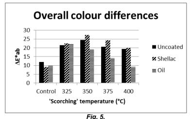
Overall colour differences for the samples, at the end of the testing phase.
