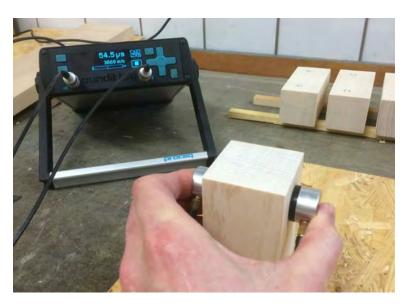
Fig. 4. Ultrasound measuring device Proceq Pundit Lab.
