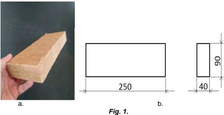
Fibre board a - fibre board; b - size of test sample 250x90x40mm.
