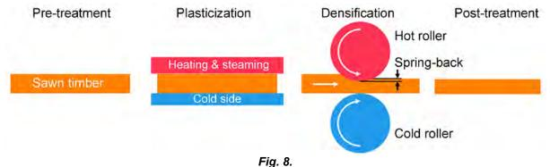
Schematic illustration of a continuous surface densification process.
