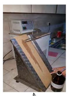
Fig. 4. Determination of the surface absorption of HDF panels: a-principle, with 1-pipette; 2-test piece; 3-inclined support; b-expermental set-up.
