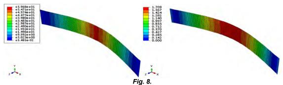
Displacements and stresses distribution in case of the modeling of an elasto-plastic material.
