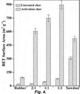
BET surface area of char from co-pyrolysis of rubber and sawdust.
