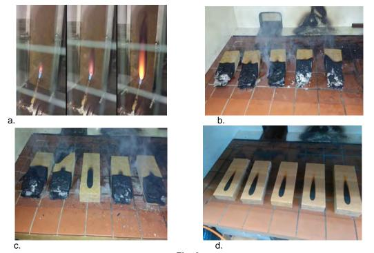
Fig. 2. Fiber board after dipping a – pre-test, b- dipping after 6 min, c – dipping after 9 min, dipping after 12min.
