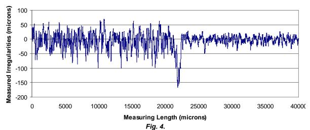
Mixed profile measuring approximately half length from beech engraved with L17 laser power at 100mm/s scanning speed and half from unprocessed beech. Profile length: 40mm.
