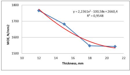
Fig. 6. Modulus of elasticity related to panel thickness.
