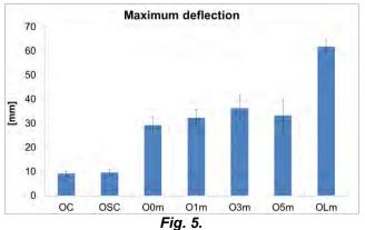
Maximum deflections for the control and the modified materials. Abbreviations: OC-control sample; OSC-steamed control sample; O0m, O1m, O3m, O5m-longitudinally compressed samples with 0, 1, 3 and 5 minutes relaxation time; OLm-compressed and long-time relaxed sample.
