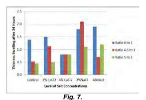
Thickness swelling of the composite samples at 24 Hour
