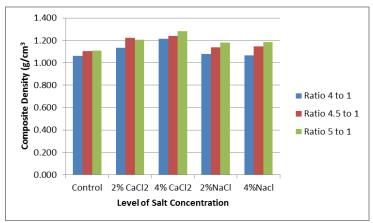
Fig. 1. The densities of the composite samples.
