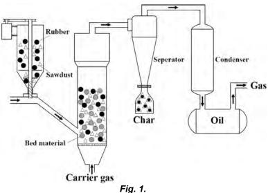
The 1 kg h<sup>-1</sup> stainless pyrolysis reactor.
