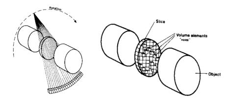
Fig. 2. X-rays emitted during rotation are being detected and then calculated to give a map of attenuation coefficients.
