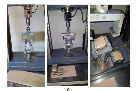
Fig. 6. Determination of the internal bond of HDF panels: a - principle: 1 – clamping device; 2 - test piece; 3 – metallic jig; F-load (tensile force); b – gluing of wooden sample on metallic jig; c - ZWICK 010 testing machine.
