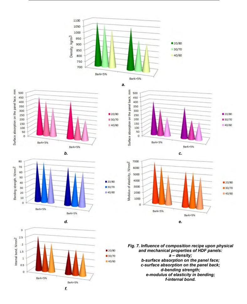
As one may notice, all mechanical properties are lowered by the use of the release agent. The lowest (worst) values were obtained when spraying with water (24.1% reduction of bending strength, 34% reduction of elasticity modulus and 40.5% reduction of internal bond) and the best when using the release agent PAT 2003 XE (by Würtz): only 6.9% reduction of bending strength and 8.4% reduction of elasticity modulus and 27% reduction of internal bond.
