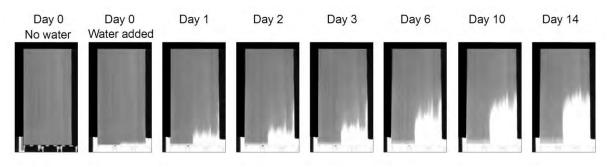
Fig. 3. Water absorption (white area) in an aspen specimen containing sapwood and heartwood in cross section view according to Fig. 1.
