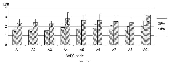
Fig. 1. Variation of Ra and Rq roughness parameters (mean values and standard deviations) with the WPC composition.
