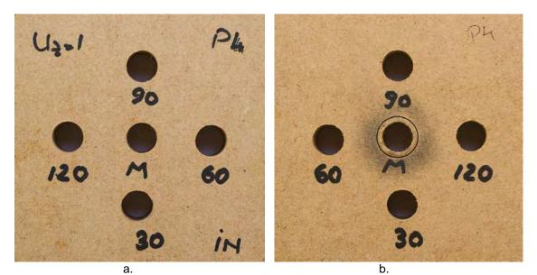
Fig.7. Sample drilled with twist drills and tooth byte  $f_z$  of 0.1 mm: a - at the entrance side b - at the exit side.
