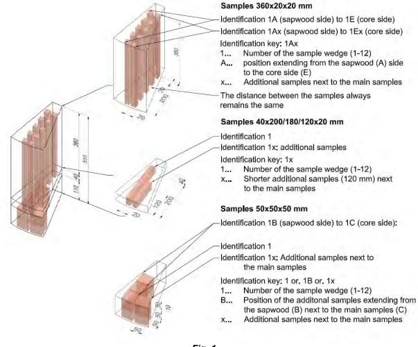
Fig. 1. Schematic description of the material preparation.
