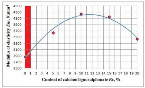
Fig. 3. Variation of modulus of elasticity of MDF in dependence from the content of calcium lignosulfonate.
