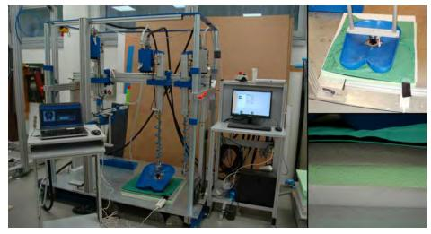
Fig. 2. Laboratory test setup with the anatomical seat load pad and layered foam structure.
