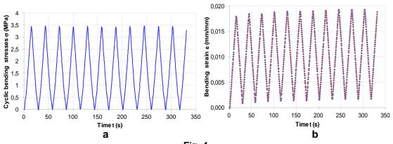
Fig. 4. Cyclic variation of bending stress (a) and (b) strain.
