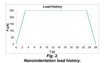
The peak load ( $P_{max}$ ) and the contact area (A) are recorded during the experiment. By dividing  $P_{max}$  by A, hardness (H) could be calculated. The indentation modulus ( $E_r$ ) is determined from the initial slope of the unloading curve (Konnerth and Gindl 2006).  $E_r$  takes into account the indenter tip's compliance. The influence of the diamond indenter's indentation modulus is negligible.
