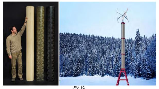
Moulded tubes from Norway spruce (left) with a length of 250 cm, a diameter of 28 cm, and a tube-wall thickness of 2 cm, and to the right a wind-power plant from fibre-reinforced moulded tube (Kutnar et al. 2015).
