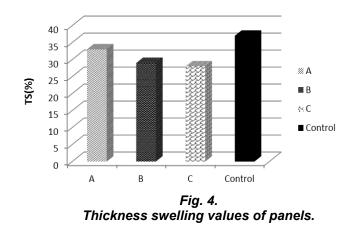
Fig. 4 shows the TS values of MDF panel samples. The tendency of TS values was found similar to the WA values. It was determined that the TS values also reduced with increasing the ratio of sawdust. The highest TS value was found to be 37,04% for control panel. The panel type C had the lowest TS value. This value was recorded to be 28,43%.
