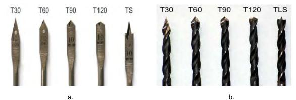
Fig. 1. Types of drills used for processing:  $a - four flat drills with the tip angle 2\kappa$ , of 30°, 60°, 90°, 120° and one spade drill; b – four helical drills with the tip angle  $2\kappa_r$  of 30°, 60°, 90°, 120° and one lip and spur drill.
