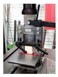
Fig. 3. Test facilities for the determination of the shear strength in longitudinal-radial (Ir) and longitudinal-tangential (It) direction according to DIN 52187.
