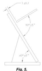
Experimental set-up for the determination of the surface absorption: 1-pipette; 2-test piece; 3inclined support.
