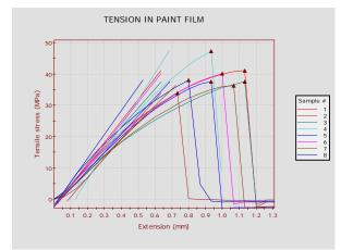
Fig. 11. Tensile tension in samples of lacquer films of polyurethane-1K.
