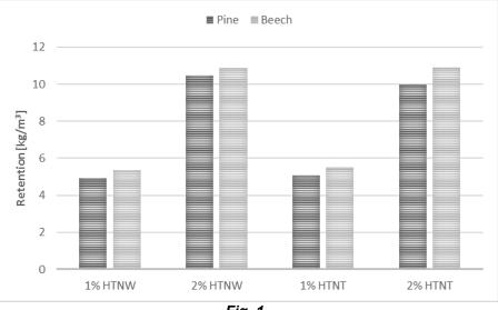
Fig. 1. Retention of nanoparticles as a result of impregnation.
