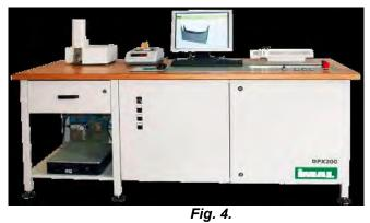
rig. 4. X-ray density profile analyser DPX300, IMAL production.
