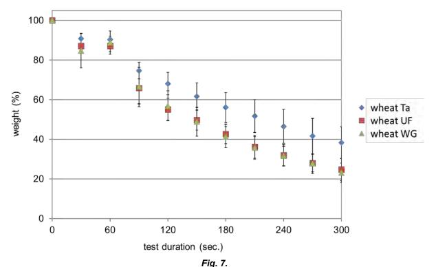
Mass change after fire test of wheat straw boards (250 kg/m<sup>3</sup>) with 3 different types of adhesive.
