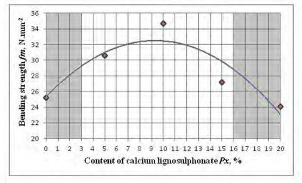
Fig. 2. Variation of bending strength of MDF in dependence from the content of calcium lignosulfonate.
