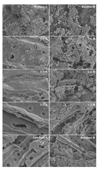
Fig. 5. SEM images of the char from co-pyrolysis of rubber and sawdust. A: untreated char; B: activated char.
