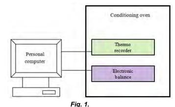
Diagram showing the instrumentation for the entire assembly.
