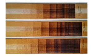
Fig. 7. The three samples at the end of the testing phase (top) uncoated (centre) shellac coated (below) oil coated.
