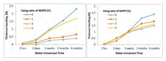
Fig. 1. Coupling agent effect on thickness swelling of the thermoplastic composites.
