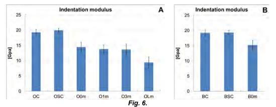
Indentation moduli of the control- and differently treated samples: A – oak; B – beech. Abbreviations: OC and BC-control sample; OSC and BSC-steamed control sample; O0m and B0m, O1m, O3m-longitudinally compressed samples with 0, 1 and 3 minutes relaxation time; OLm-compressed and long-time relaxed sample.
