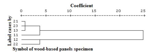
Fig. 1. Cluster analysis of the wood-based panels based on the degradation grading values. Wooden products specimen symbol is present at Table 2.
