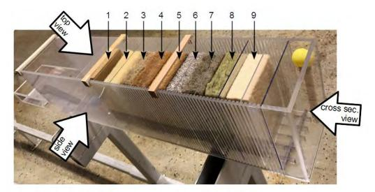
Fig. 1. Experimental setup. Tested bio-based insulation material in the rig are: (1) Pavatherm combi (wood fibers), (2) Glass fiber, (3) Thermohanf Premium (hemp), (4) Thermojute (jute), (5) STEICOflex (pine wood fibers), (6) iCell (newspaper), (7) Isolina (linen), (8) Stone wool, (9) Thermocell (pulp).
