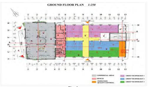
Fig. 6. Rearranged of machines into GT.
