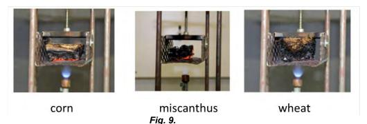
Visual changes of the insulation boards after the 300 seconds of the fire test
