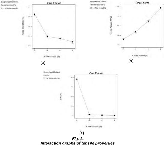
a) tensile strength, b) tensile modulus & c) elongation at break.
