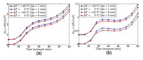
Fig. 3. Energy release rate versus time and different crack tip advance ( $\Delta a$  =1 mm and  $\Delta a$  =8 mm), for mixed mode during heating process ( $\Delta T$  =+20°C): Open mode part (a), Shear Mode part (b).
