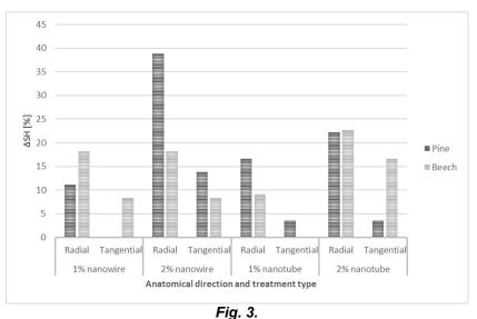
Decrease in the shrinking coefficient as a result of nanoparticle treatment.
