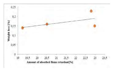
Fig. 5. Graph of the amount of absorbed retarder in percentage and its weight loss after 12 minutes of soaking.
