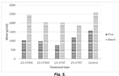
Water uptake during 72 hours immersion in water in radial direction.
