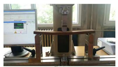
Fig. 4. IMAL model IBX 600 equipment for determination of MOR and MOE.
