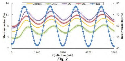
Moisture content changes where RH changes sinusoidally at a constant temperature against cyclic time for poplar wood with different treatments (cyclic period of 24 h).
