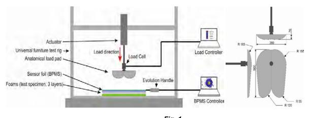
Fig. 1. The schematic principle of measurements and the geometry of the loading pad.
