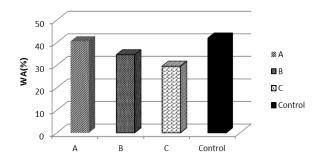
Fig. 3. Water absorption values of panels.
