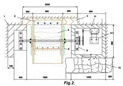
Longitudinal section through the concrete structure, turbine and wooden spouts – Principial scheme - Variant 2 including a generator unit 1 –edged concrete structure; 2 –fast/ immobile wooden spout 3 – water flow rate; 4 – log barrage; 5 –mobile spout; 6 – generator unit ; 6.1 –consumer; 9 - bearings; 11 – concrete structure.
