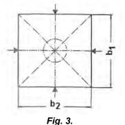
Measuring the dimensions of the test pieces for HDF density determination.
