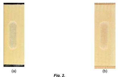
PMMA/ATH + PF coating after 1000 cycles on glass (Fig. 2a) and wood (Fig. 2b).
