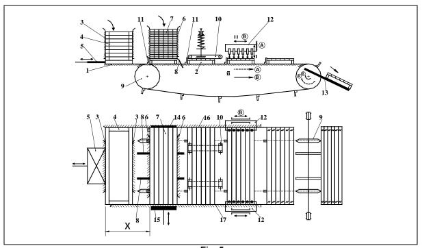
Fig. 5. Equipment of panelling the frames with close or spaced lamellas.
