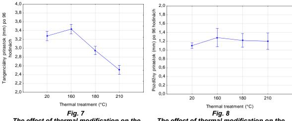
The effect of thermal modification on the tangential gain during soaking
