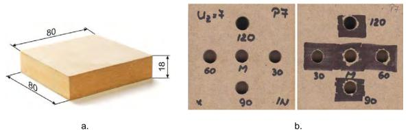
Fig. 2. Samples used for drilling: a – sample dimensions; b - MDF specimens drilled with the flat drills (T30, T60, T90, T120, TS) when the tooth bite was 0.7 mm at the entrance side and the exit side.
