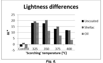
Overall lightness differences for the samples, at the end of the testing phase.
