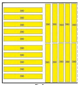
Fig. 2. Sampling of solid wood panels for bending test.
