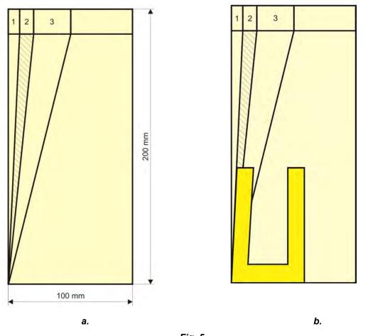
Fig. 5. Determination by means of fork-samples of the internal stresses caused by drying: a – evaluation jig; b – correct positioning of the fork-sample on the jig.
