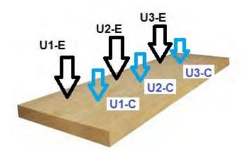
Fig. 2. Assessing the moisture content of the timber boards, as average of six values, measured over timber length (1-2-3), in central part (C) and exterior part (E) of the board.
