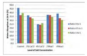
Fig. 5. Water absorption by the composite samples at 24 Hour.
