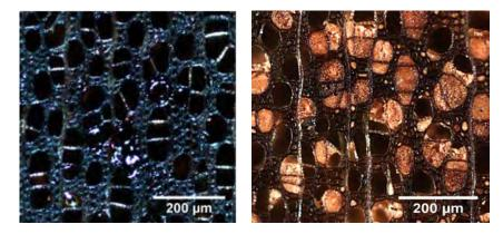
Fig. 4. Surface images of poplar impregnated with 50% pyrolysis liquid (left; Pyrol\_Can) and sample after leaching & post-vacuum (right). Photos: R. Rousek.
