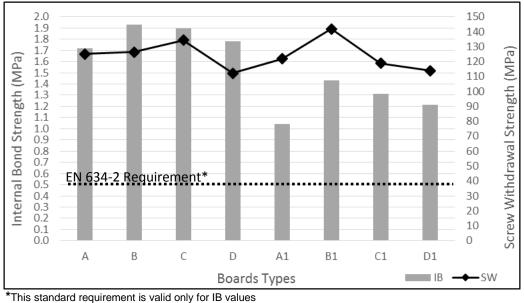
Fig. 2. Properties of IB and SW strength of the boards.
