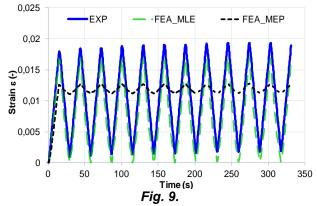
Strain variation - experimental and numerical determinations.
