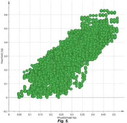
Observed (vertical axis) and predicted (horizontal axis) volume yield according to the PLS model.
