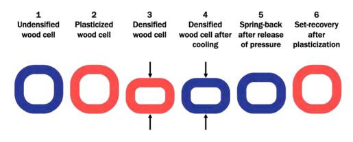
Fig. 6. Cross-sectional view of a wood cell showing the nature of set-recovery and spring-back.
