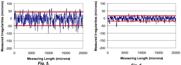
Detail of the mixed profile from Fig. 4., representing only the laser scanned region (left part) of the profile (laser power L17 and 100mm/s scanning speed). The red lines represent thresholds delimiting the core roughness. Profile length: 20mm.
