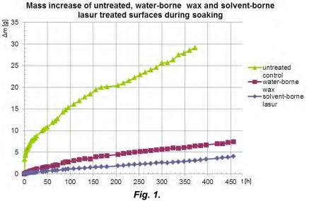
Mass increase of untreated, water-borne wax and solvent –borne lasur treated surfaces during soaking.
