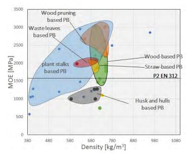
Fig.10. Ashby plot of alternative particleboard's MOE, and panel density.
