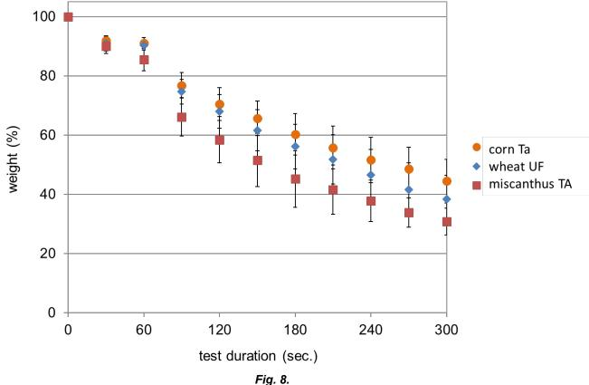
Mass change of the various insulation boards (250 kg/m<sup>3</sup>) during fire test.
