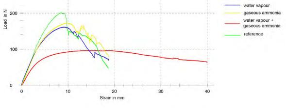
Fig. 3. Load-displacement curves for treated and reference samples.
