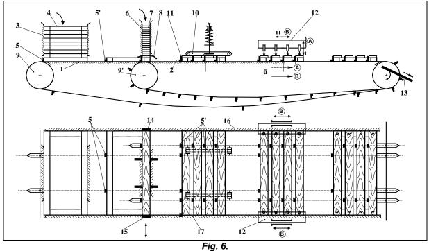
Equipment for forming wooden framed panels for crates by using frames and spaced lamellas.
