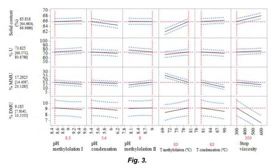
Reaction parameters as a function of resin properties.
