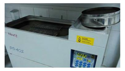
Fig. 4. NUVE-BS402 equipment used for the determination of the swelling in thickness after water immersion of the tested particleboards.
