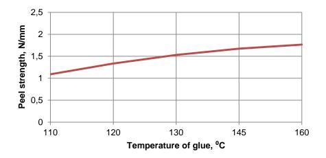
Fig. 4. Relationship between peel strength of glue joint and temperature of glue during through feed lamination of particle board with PVC foil.
