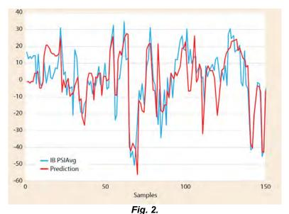
Illustration of real-time predictions of "IB" (internal bond) of wood composites.
