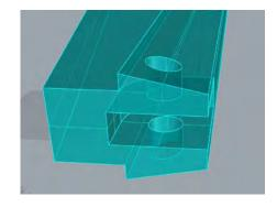
Fig. 3. Dovetail female joint of the beam/rafter at eaves node.
