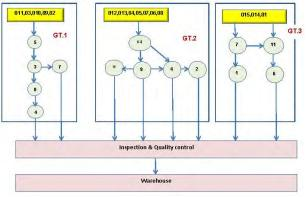
Fig. 5. Flow diagram of parts in rearranged GT.
