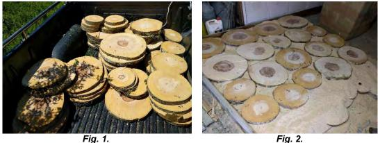
View of the collected beech stem discs. Storage of stem discs for indoor air-dry.
