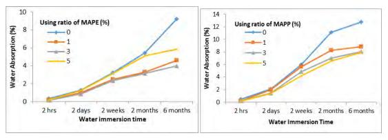
Fig. 2. Coupling agent effect on water absorption of the thermoplastic composites.
