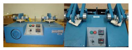
Fig. 1. Taber equipment used for the abrasion test.
