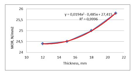
Fig. 5. Slight influence of thickness on static bending strength.
