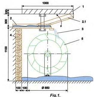
Cross section through the barrage, turbine, wooden spouts and bridge sustaining the mobile spout- Principial scheme 1 – bridge sustaining the mobile spout; 2 – fast spout; 2.1 –mobile spout 3- water flow rate; 4 – logs barrage; 5 – turbine.
