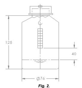
Principle of determining the formaldehyde emission from particleboards by means of the flask method.
