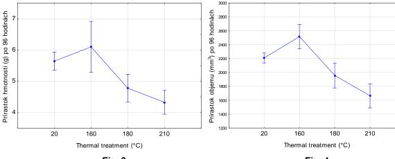
Fig. 3 The effect of thermal modification on the weight gain during soaking
