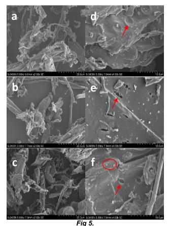
Scanning electron micrographs of pyrolysis residues at different magnifications (2.00k and 4.00k): (a) and (d) untreated samples; (b) and (e) Soxhlet extracted samples; (c) and (f) ultrasound-extracted samples.
