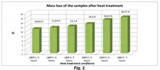
Mass loss of the samples after heat treatment.
