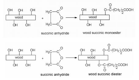
Fig. 1. Chemical modification of wood samples - Possible reactions.
