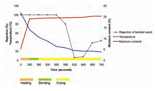
Fig. 4. Temperature, moisture content and rejection as a function of time during the bending of solid beech wood using dielectric heating.
