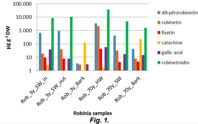
Analysis of methanol – water 1:1 extracts from Robinia (Rob): Influence of age (years; sapwood SW, heartwood HW), and stem compartment (inner and outer parts of disc, Wood or Bark) on amount of flavonoids and phenolic compounds.
