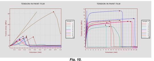
a –Tensile tension in samples of lacquer films b polyurethane-2K.
