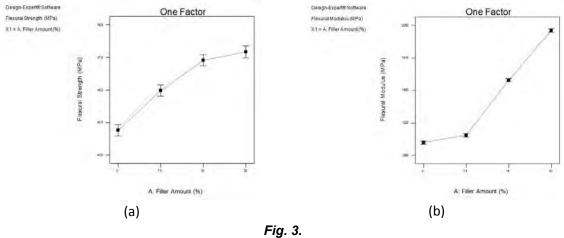
Fig. 3. Interaction graphs of flexural properties a) flexural strength & b) flexural modulus.
