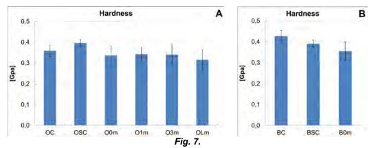
Hardness of the control- and differently treated samples: A – oak; B – beech. Abbreviations: OC and BC-control sample; OSC and BSC-steamed control sample; O0m and B0m, O1m, O3mlongitudinally compressed samples with 0, 1 and 3 minutes relaxation time; OLm-compressed and long-time relaxed sample.
