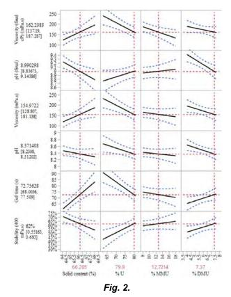
Resins quality measurement as a function of resin properties.
