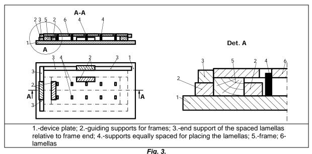
Technological device designed to position the spaced lamellas for their consolidation on the frame.
