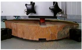
Fig. 4. Disc surface milling with the fly cutter.
