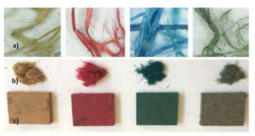
Fig.3. a) Microscopic images of the fibers b) uncoloured/coloured fibers c) uncoloured/coloured MDF samples.
