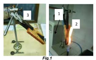
Device used in the fire experiments 1-scale, 2-sample, 3-device for clamping the specimen above the flame
