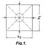
Measuring the dimensions of the particleboard samples for density determination.
