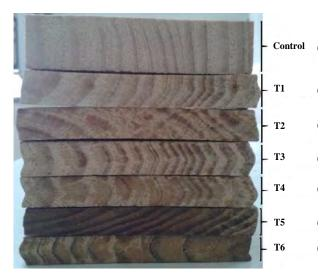
Fig. 2. View of the thickness and the shape of the board after the thermomechanical treatments.
