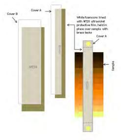
Fig. 4. Natural light aging, sample preparation plan (Millis 2012, Millis 2013).
