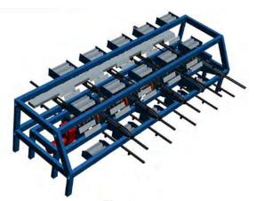
Fig. 2. Board scanner with traditional vision system and laser-based tracheid measurements (Illustration by RemaSawco).
