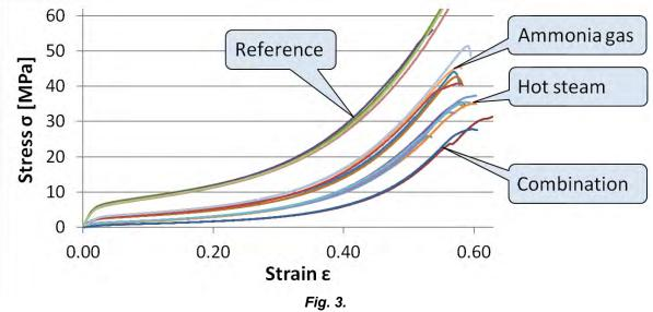
Stress-strain relationship for tangential compression of untreated beech (reference) and beech softened by ammonia gas, saturated steam or both in combination (Rousek et al. 2015).
