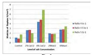
Fig. 3 The Modulus of Rupture of the composite samples.
