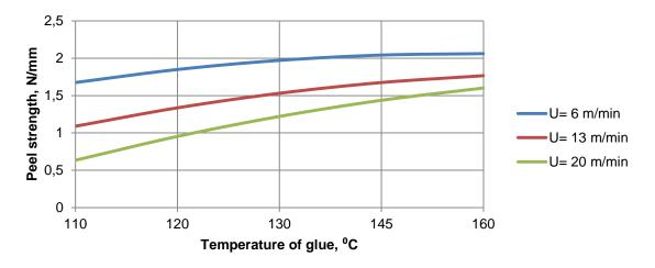
Fig. 5. Relationship between peel strength of glue joint, feeding speed and temperature of glue during through feed lamination of particle board with PVC foil.
