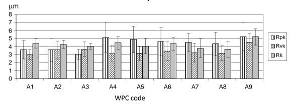
Fig. 2. Variation of Rpk, Rvk and Rk roughness parameters (mean values and standard deviations) with the WPC composition
