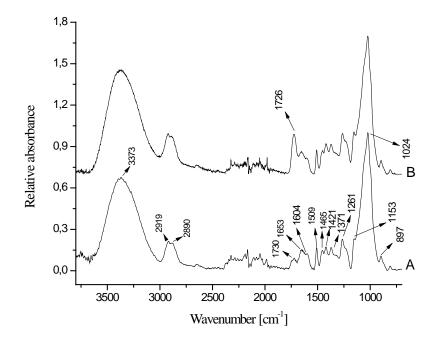
Fig. 1. FT-IR spectra: (A) etalon sample (Abies alba wood); (B) sample 3 (Abies alba wood sample esterified with succinic anhydride).
