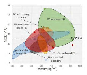
Fig. 9. Ashby plot of alternative particleboard, showing MOR along with panel density.
