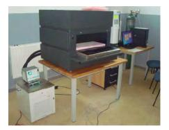
Fig. 1. HFM 436 Lambda heat flow meter used for thermal conductivity determination
