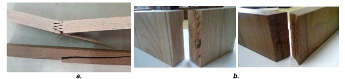
Fig. 5. Rupture caused by static bending in panel sample: a-longitudinal sample; b-transversal sample.
