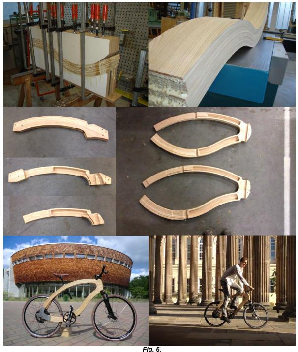
Selected manufacture steps of the Wooden E-Bike: lamination of 5 mm thick ash boards to a "glulam" component (upper), CNC milled bicycle components (middle), and the finished E-Bike in use.
