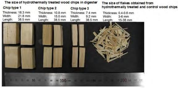
Fig. 1. The sizes of wood chips used for the hydrothermal treatment.
