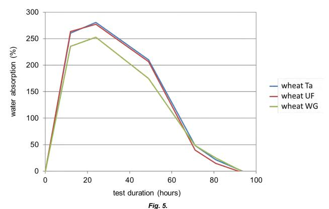
Influence of different adhesives on wheat straw boards (250 kg/m³) on the water absorption and water release.
