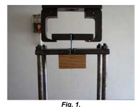
Samples used in tests to determine withdrawal capacity of screws in radial direction.
