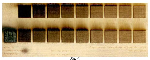
Colour scale produced of sycamore showing the effect of speed on wood colour.
