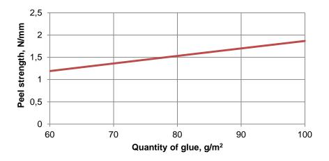
Fig. 3. Relationship between peel strength of glue joint and quantity of glue during through feed lamination of particle board with PVC foil.
