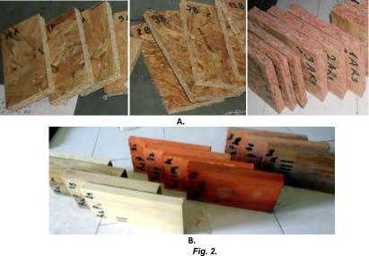
A. OSB treated samples: softwood treated samples
