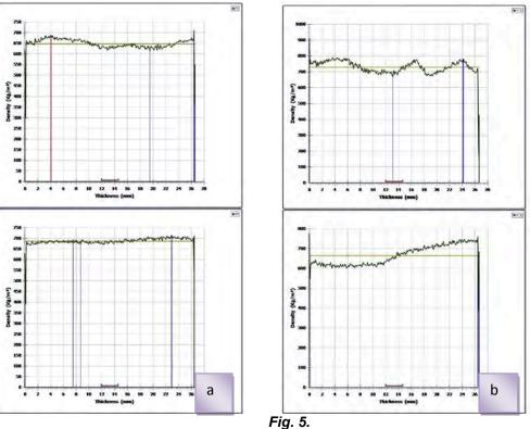
Determination of density values and density profile was carried out on specimens of 50m x 50m. X-ray density profile analyser DPX300, IMAL production has been used as equipment.
