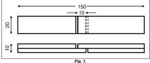
Shear strength test sample (size given in mm)
