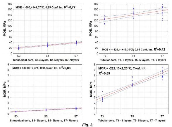
Scatter plot diagrams with regression lines of the modulus of rupture and modulus of elasticity in function of core geometry and number of veneer layers.
