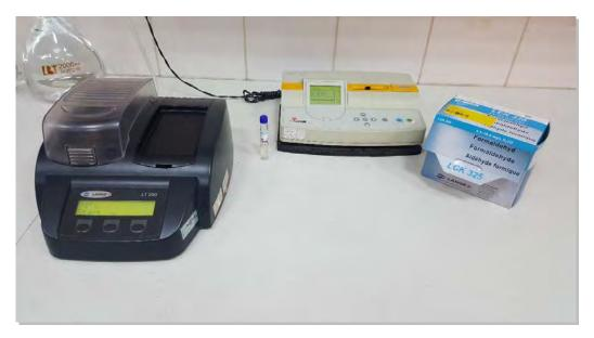
Fig. 3. Equipment for the determination of the formaldehyde emission by the flask method.
