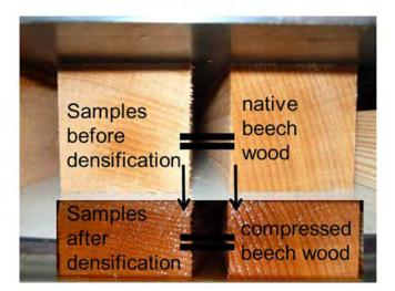
Fig. 7. The Lignamon process delivered material with improved properties (upper) compared to control and steamed-densified beech (lower), Photo: Martin Brabec.
