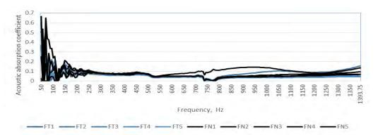
Fig. 6. Acoustic absorption coefficient of treated ash wood samples (FT1...FT5) and non-treated ash wood samples (FN1....FN5).
