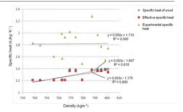
Fig. 2. Experimental and calculated effective specific heat of radially drilled briquettes as a function of density for MC  $\leq$  EMC.
