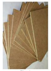
Fig. 1. Raw high-density fiberboards.
