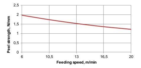
Fig. 2. Relationship between peel strength of glue joint and feeding speed during through feed lamination of particle board with PVC foils.
