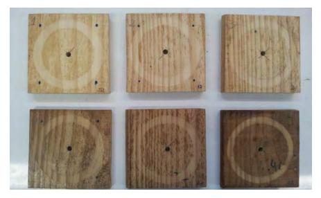
Fig. 4. Apperance of the samples after the abrasion test.
