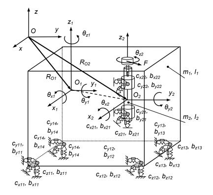
Fig. 3. Mechanic-mathematical model of the wood shaper and its spindle.
