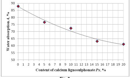
Fig. 2. Variation of water absorption of MDF in dependence from the content of calcium lignosulfonate.
