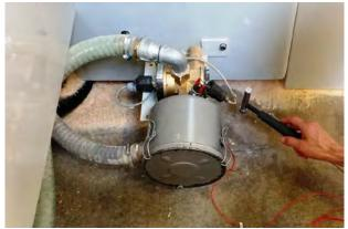
Fig. 3. Measuring point at the upper rear machine foot of the CNC machine.
