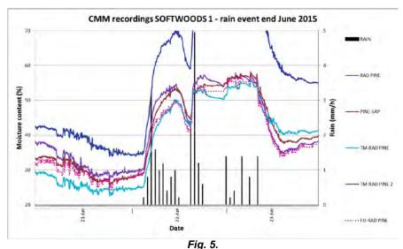
Field test moisture recordings (CMM) of softwoods with high absorption.
