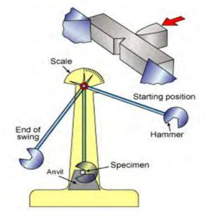
Fig. 2. Charpy pendulum impact machine (IT 2017).
