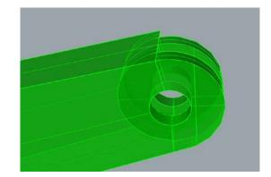
Fig. 1. Dovetail male joint of the beam/rafter at eaves node.
