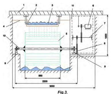
Longitudinal section through the bridge- Principial schema Variant 1- with alternator
