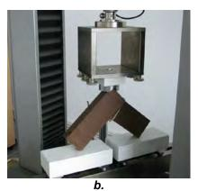
Fig. 3. Testing of end to edge butt joint at compression (a) and tensile (b).
