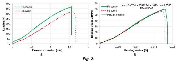
Load-displacement (a) and stress-strain (b) functions under static bending.
