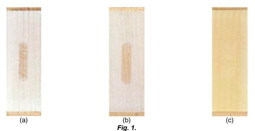
Coating after 1 cycle. (a): sample  $A_w$  (PMMA/ATH with compressed air); (b): sample  $B_w$  (PMMA/ATH with forming gas); (c) sample  $C_w$  (PMMA/ATH + PF with compressed air).
