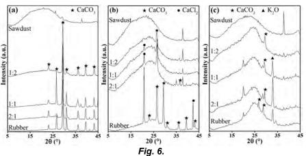
X–ray diffraction of the char from co-pyrolysis of rubber and sawdust. (a) Untreated char; (b) Demineralized char; (c) Activated char.
