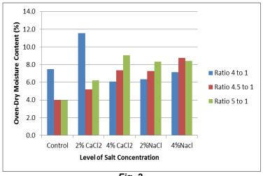
Fig. 2. The oven dry moisture contents of the composite samples
