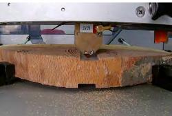
Fig. 5. Disc surface scanning with the high frequency probe.
