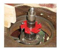
Fig. 2. Spindle with bearing units and with cutter.
