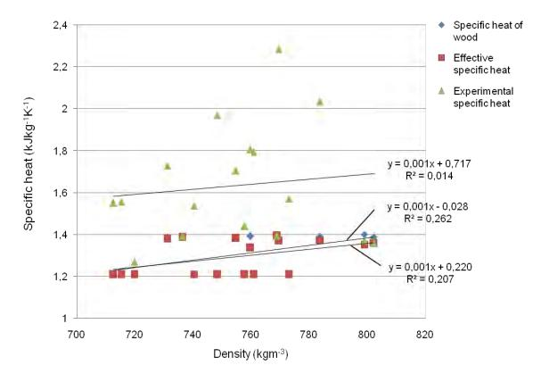
Fig. 1. Experimental and calculated effective specific heat of longitudinally drilled briquettes as a function of density for  $MC \le EMC$ .
