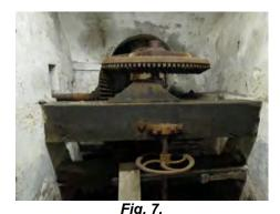
The turbine producing electricity: the teeth of the upper gear are made of service tree wood.
