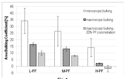
Fig. 1. Area bulking coefficient (ABC) of the PF treated beech cell walls (microscopic bulking) and of PF treated beech blocks (macroscopic bulking) at a PF concentration of L-PF 45%, M-PF of 45% and H-PF 45% and wood blocks at 20% PF concentration (macroscopic bulking – 20% PF concentration).
