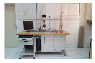
Fig. 6. IMAL IB600 equipment used for the determination of the bending strength and modulus elasticity in bending of the tested particleboards.
