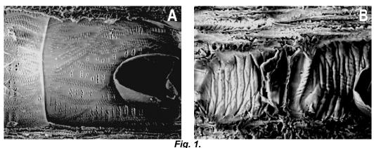
SEM photographs of the oak wood's trachea in case of 2 samples (20 kV x200): A – control; B – longitudinally compressed.
