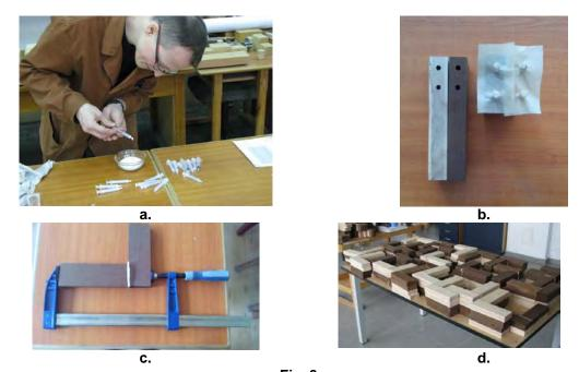
Fig. 2. Dispensing the adhesive (a), applying the wax paper (b), pressing the parts of joint (c) and conditioning the joints (d).
