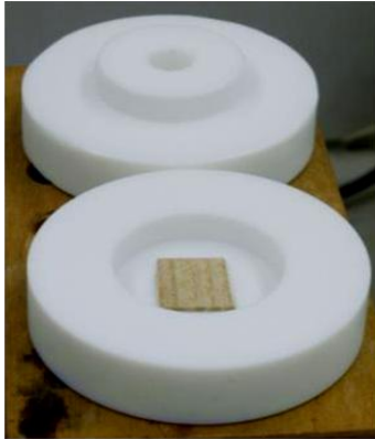
Figure 1. Teflon container with inserted veneer
