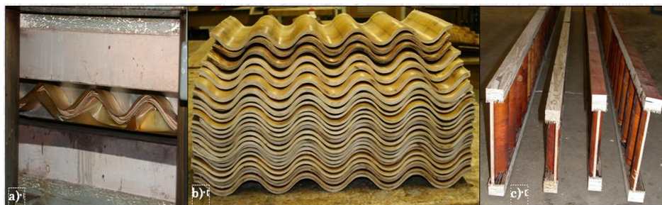
Figure 1. a) Corrugated press templates; b) Web panels with different thicknesses; c) Prefabricated I-joists
