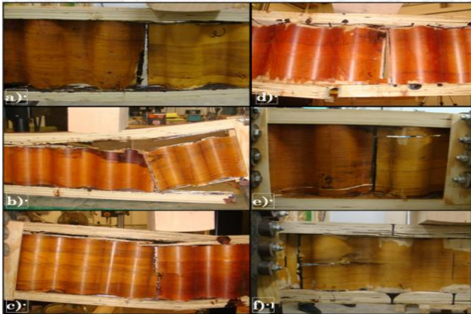
Figure 2. Typical joist failures
