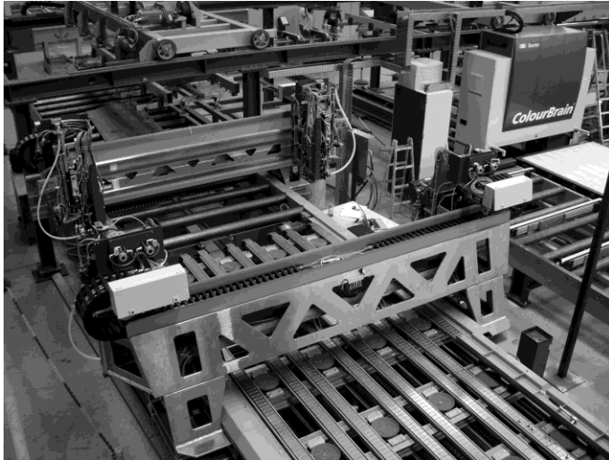
Figure 3. The panels are scanned by the multi-sensorial ColourBrain® scanner (right top) before entering the complex automatic patching plant with several NC patching tools operating in parallel
