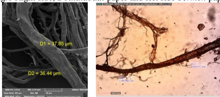
Fig.2 Morphology and dimensions of fibers, right side with Optical Microscope (OM) and left side with Scanning Electron Microscope (SEM)
