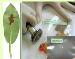
Fig. 4: Leaf tissue disruption by Mesh Bag homogenization
