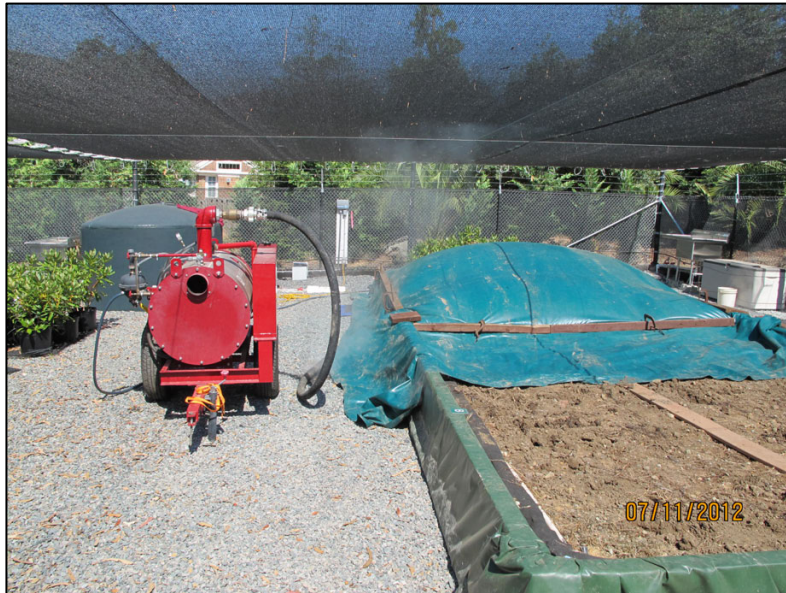
Figure 1: Steam sterilization of a research plot at NORS-DUC using a SIOUX Steam Flo SF-11 unit.
