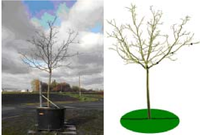
Fig. 1: Walnut tree, left: general features, right: digitized geometry; the dots show the position of displacement sensors
