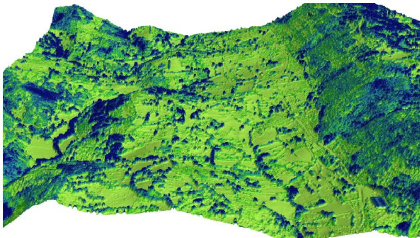
Air-borne lidar-based information can be considered from the beginning of a forest inventory supporting the set-up of multistage/multiphase sampling designs (i.e. lidar data acquisition is conceived as a part of the sampling design) or just after the end of the field survey, prevalently to support small area estimations, wall-to-wall mapping or the treatment of missing field data.
