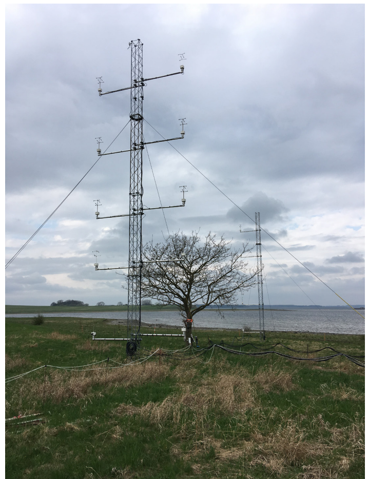
Oak tree at Risø campus, Roskilde, which is monitored for movement in the wind. Masts are instrumented with sonic anemometers to measure the flow in front of and behind the tree. Copyright: Barry Gardiner, EFI
