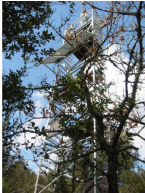
Photo: Eddy-correlation tower for measuring canopy-level ozone flux in a Mediterranean forest (provided by IUFRO RG 7.01.00)
