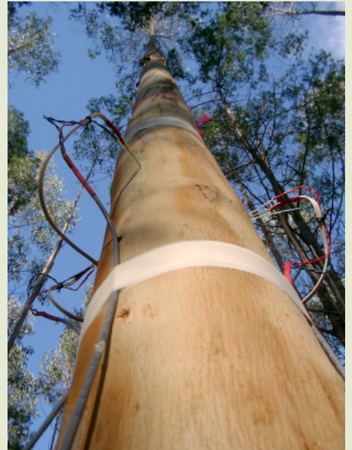
Measuring transpiration by collecting sap flow data from a Eucalyptus globulus tree that is growing in a mixed species plantation with Acacia mearnsii. This will be used to under-stand the processes driving species interactions in these mixtures. (Photo by David Forrester; Cann River, Australia)
