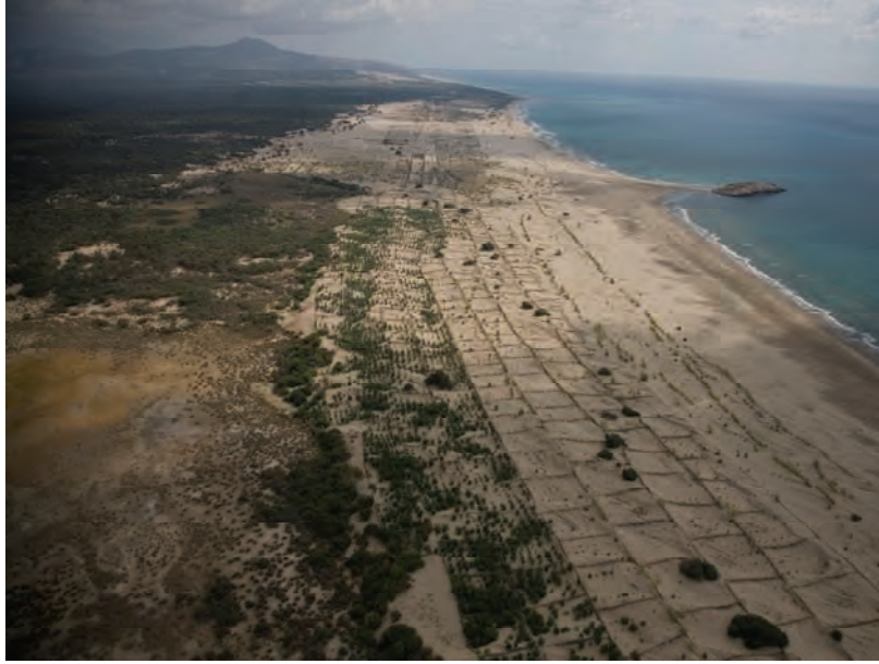
Different phases of sand dune stabilization work in the Mediterranean Region (Photo taken by A. INCE)
