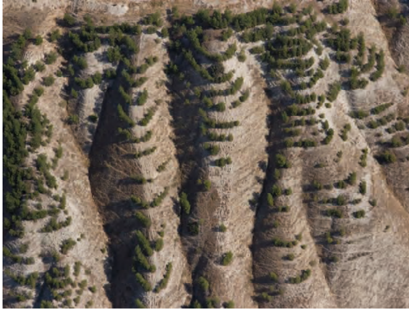
Erosion control with terracing by using coniferous species in South-eastern Turkey (Photo taken by A. INCE)
